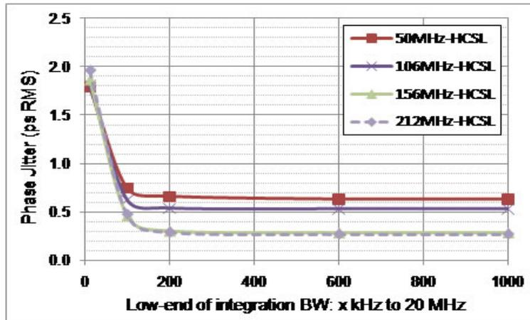
Figure 1. HCSL Phase Jitter (integrated phase noise)
