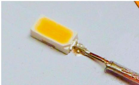
Figure 5. Photo showing actual placement of TC wire secured with thermal conductive epoxy. The thermal epoxy volume should be kept to minimum as shown.
