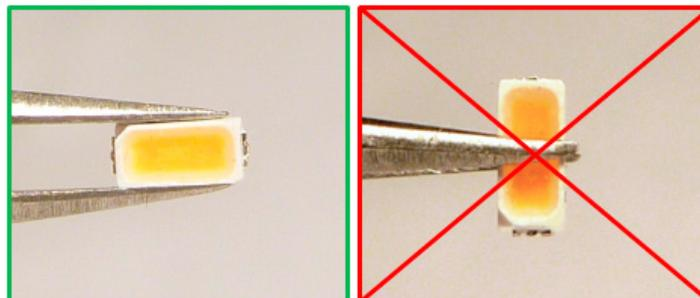
Figure 2. Correct handling (left) and incorrect handling (right) of LUXEON emitters.
