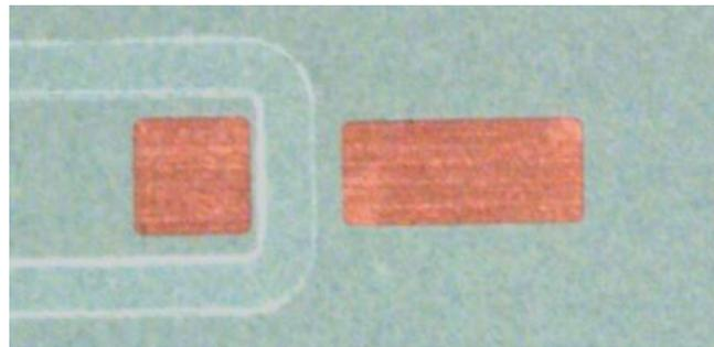
Figure 3. Recommended PCB footprint design for the LUXEON emitter (top). In order to ensure proper heat dissipation from the package electrodes to the PCB, it is best to extend the top copper layer of the PCB several millimeters beyond the package of the LUXEON emitter. See Section 3 for more information on the copper layout. All dimensions are in mm. Bottom picture shows the actual FR4 PCB footprint layout.
