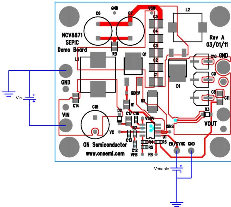
Figure 2. Evaluation Board Connections
