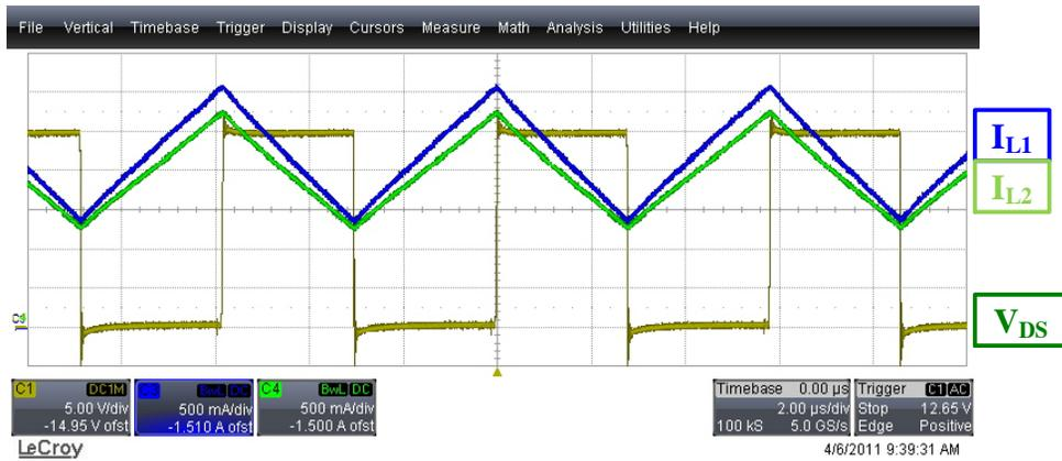
Figure 4. Operational Waveforms,  $V_{IN} = 12\text{ V}$ ,  $R_{OUT} = 6\ \Omega$
