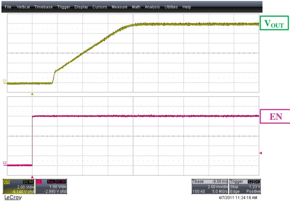
Figure 3. Typical Start-up with  $V_{IN} = 12\text{ V}$ ,  $R_{OUT} = 6\ \Omega$
