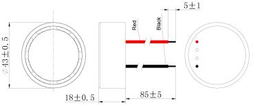
General tolerance = ±0.5 mm and all measurements in mm unless otherwise noted.
