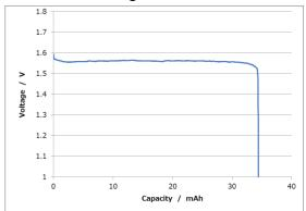
Measurement conditions: Temp: 23 deg C Load:  $20k\Omega$
