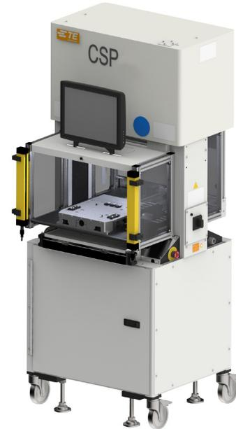
The system ensures part presence and then shuttles the product under the ram mounted upper tool to complete the press cycle. This allows the system to automatically press the product while the operators hands are free to perform other tasks such as preparing the next product to be applied. The end result is increased quality by assuring proper product location and decreased processing time.
