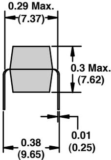
Circuit board pin spacing viewed from component side
