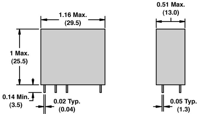
Circuit board pin spacing
