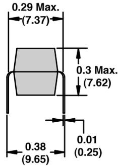
Circuit board pin spacing
