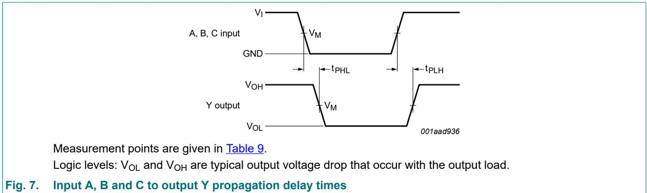
**Fig. 7. Input A, B and C to output Y propagation delay times**
