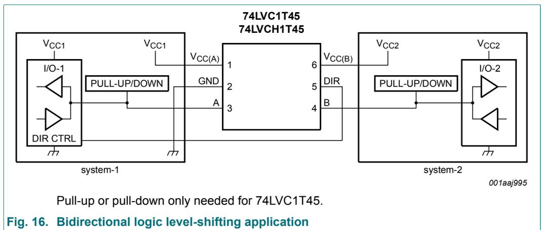
Fig. 16. Bidirectional logic level-shifting application
