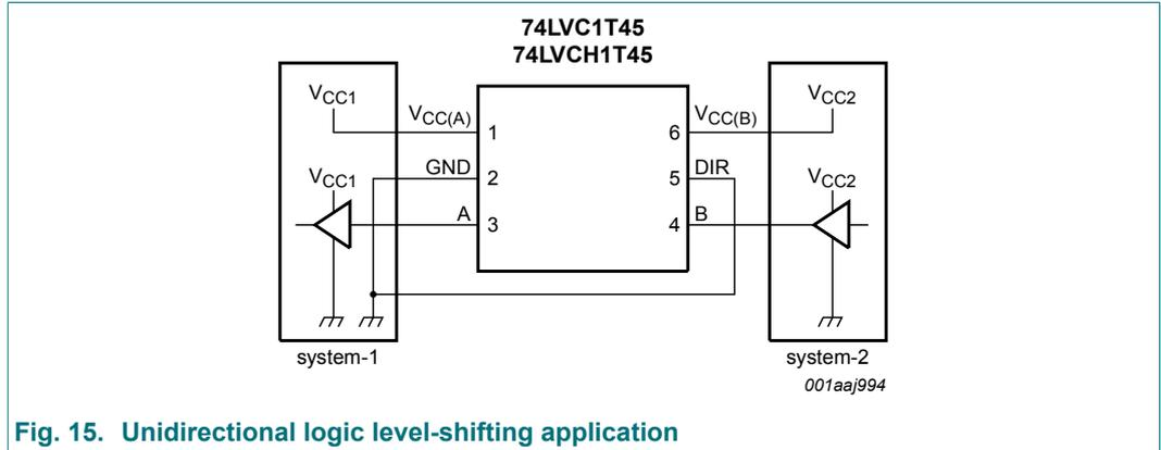
Fig. 15. Unidirectional logic level-shifting application
