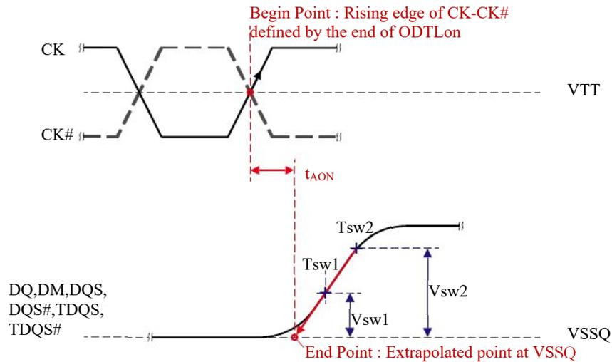
Figure 5.9.2.2 Definition of  $t_{AONPD}$
