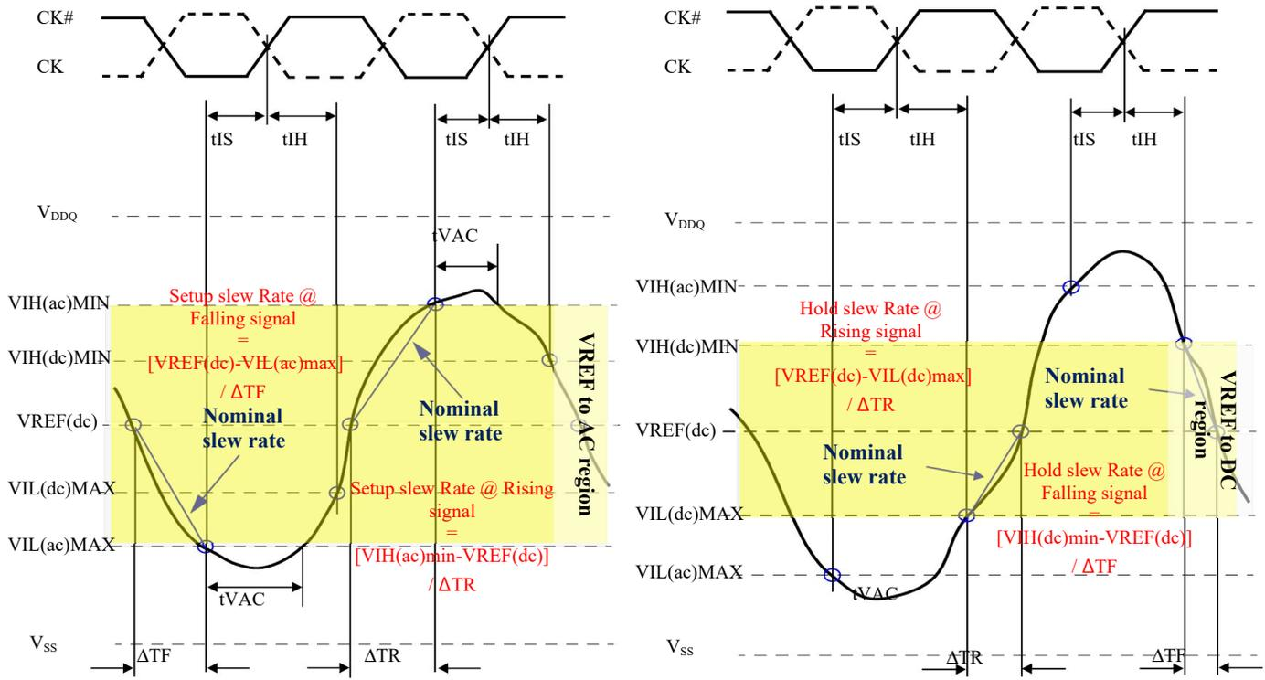
9.5.10.2 Tangent line for setup time tIS(left) and hold time tIH(right) - ADD/CMD with respect to clock
