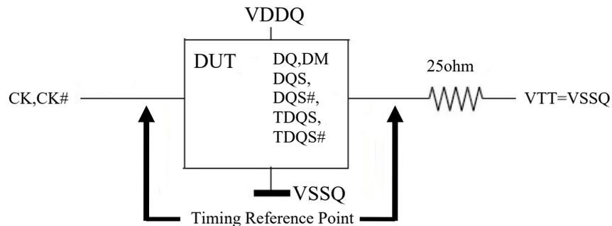
Figure 5.9.1 ODT Timing Reference Load
