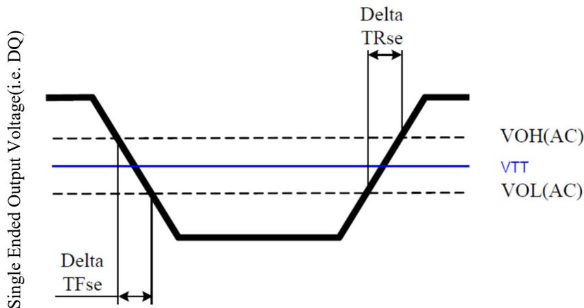
Figure 5.3.1 Single Ended Output Slew Rate Definition
