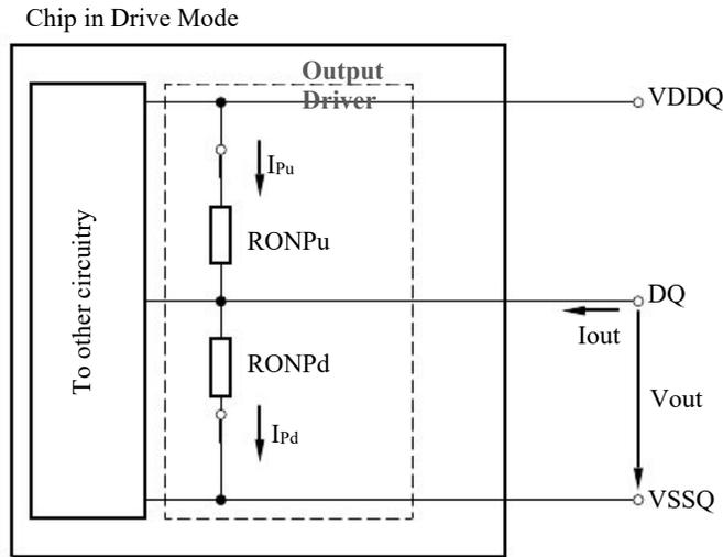
Figure 5.7 Output Driver : Definition of Voltages and Currents
