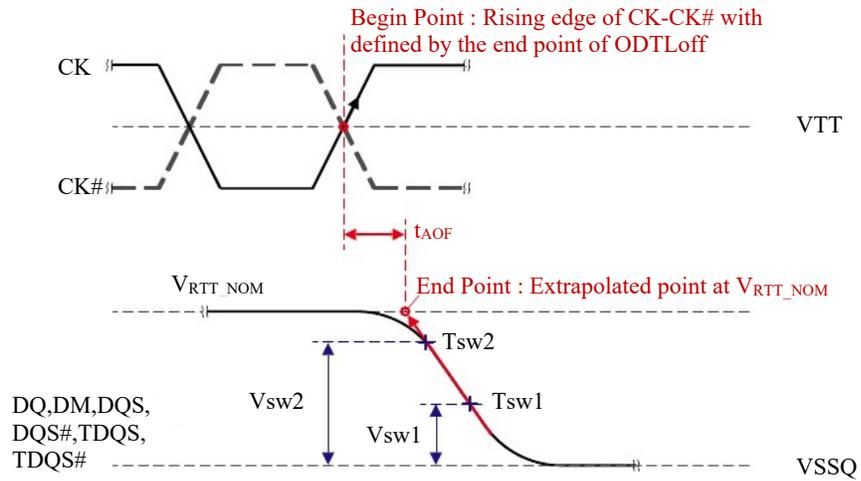
Figure 5.9.2.4 Definition of  $t_{AOFDP}$
