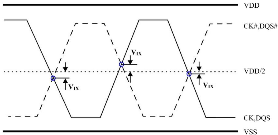
Figure 4.4.  $V_{ix}$  Definition
