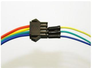
You can press wires directly into the plug connector. This works best with breadboarding jumper wires or solid-core (not stranded) copper wire.
