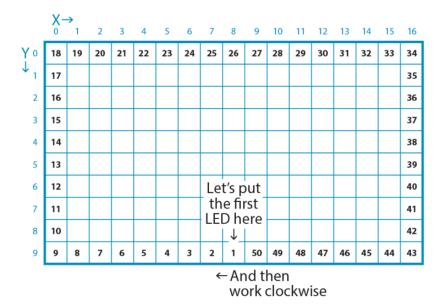
(This is the view from the <u>front</u> of the screen. When installing the LEDs on the back, you'll want to mirror the layout, flipping everything left-to-right.)
