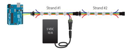
Wiring for 75, 100 or more LEDs is a little more complicated. You'll need some additional wire for distributing power, and a bit of soldering may be required.
