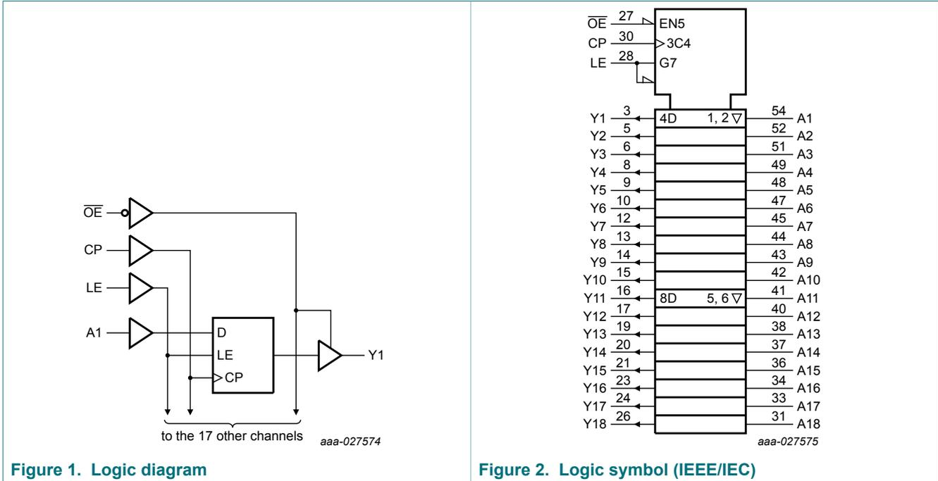
Figure 1. Logic diagram
