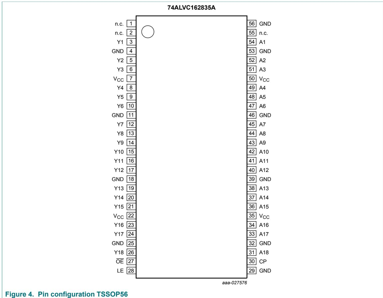
Figure 4. Pin configuration TSSOP56
