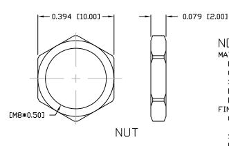
NOTE: MATERIAL HOUSING: PBT UL94V-0, BLACK CONTACT: BRASS SHELL BRASS BRASS NUT: □-RING: EPDM, BLACK FINISH: CONTACT: GOLD PLATED □VER 504" NICKEL SHELL: NICKEL NICKEL NUT:
