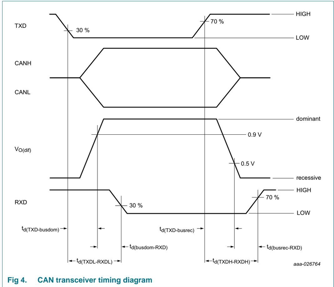
Fig 4. CAN transceiver timing diagram
