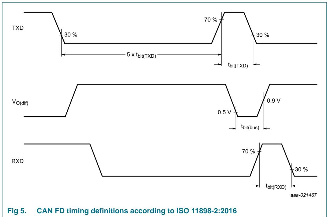
Fig 5. CAN FD timing definitions according to ISO 11898-2:2016
