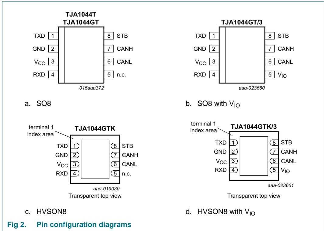
Fig 2. Pin configuration diagrams
