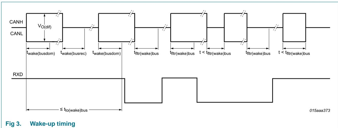
Fig 3. Wake-up timing
