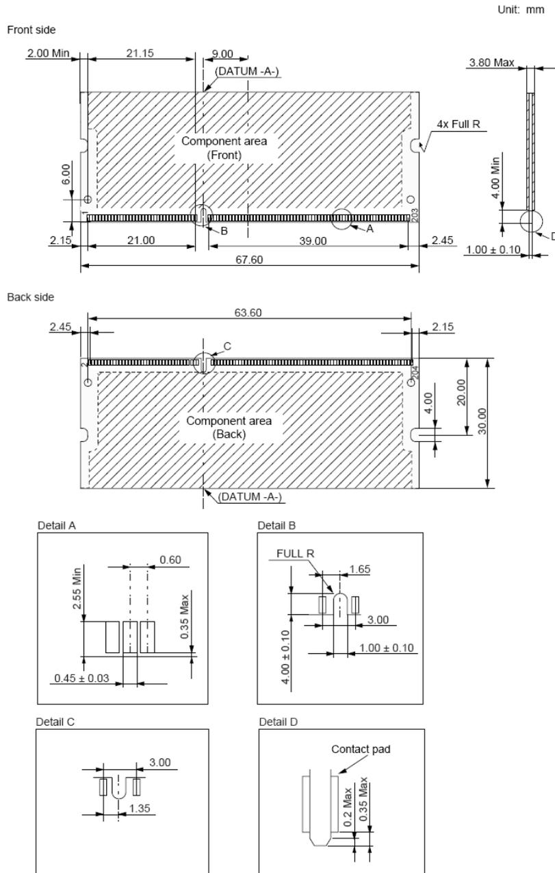
(All dimensions are in millimeters with ±0.15mm tolerance unless specified otherwise.)
