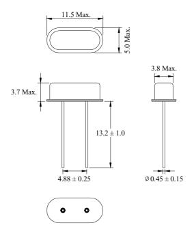
Package is Seam Sealed Ceramic-Metal. Dimensions are millimeters.
