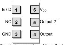
Terminations as viewed from the Top NOTE: XPRESSO LVPECL XOs are designed to fit on Industry Standard, 6 pad layouts
