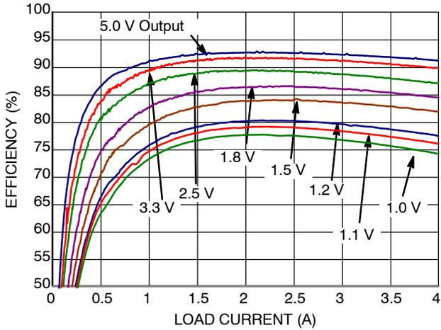
Figure 11. Efficiency ( $V_{IN} = 12\text{ V}$ ) vs. Load Current
