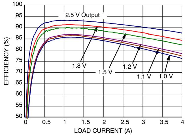
Figure 12. Efficiency ( $V_{IN} = 5\text{ V}$ ) vs. Load Current
