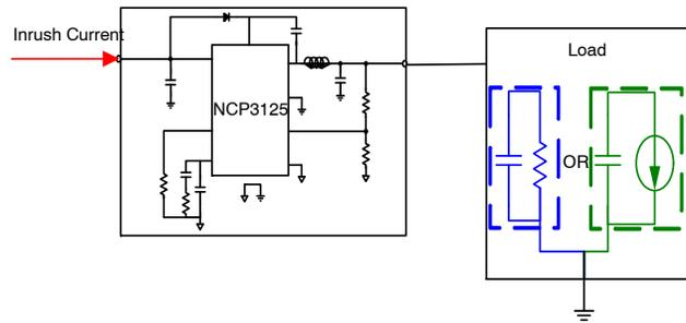
**Figure 27. Load Connected to the Output Stage**
