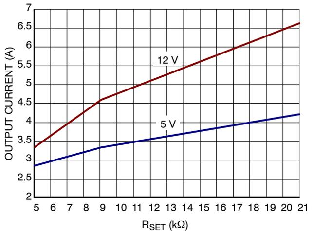
Figure 19. R<sub>SET</sub> Value for Output Current
