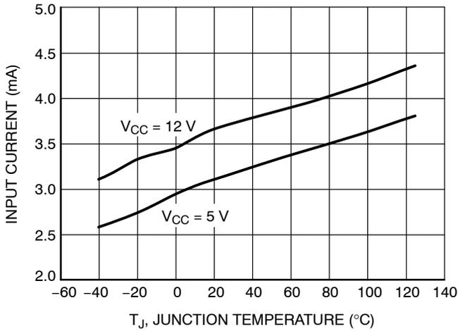
Figure 4. I<sub>CC</sub> vs. Temperature
