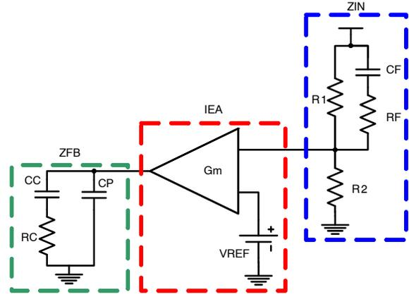
**Figure 23. Pseudo Type III Transconductance Error Amplifier**
