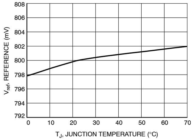
Figure 7. Reference Voltage (V<sub>ref</sub>) vs. Temperature
