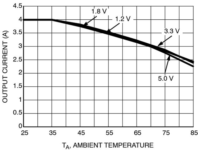
Figure 13. Derating Curve 5 V/6 V Input
