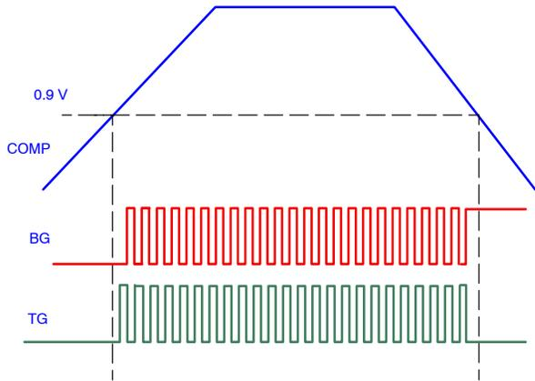
Figure 17. Enable/Disable Driver State Diagram
