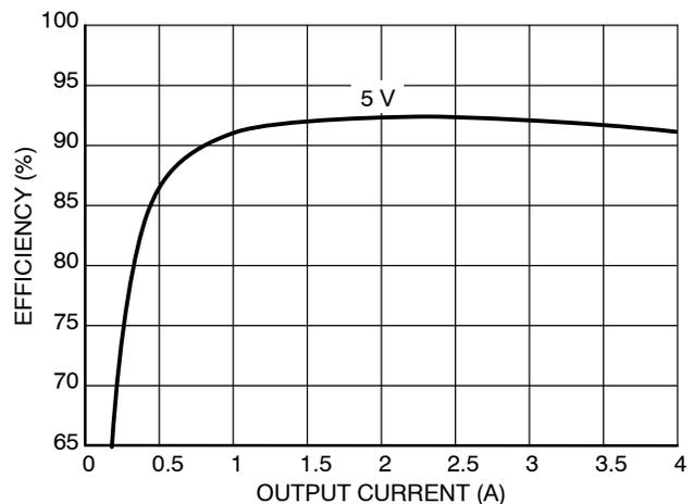
Figure 2. Efficiency ( $V_{IN} = 12\text{ V}$ ) vs. Load Current
