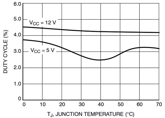
Figure 9. Minimum Active Duty Cycle vs. Temperature
