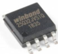
Serial Flash Memory - W25Q32FV (32Mb, 104MHz, SOIC-8)
