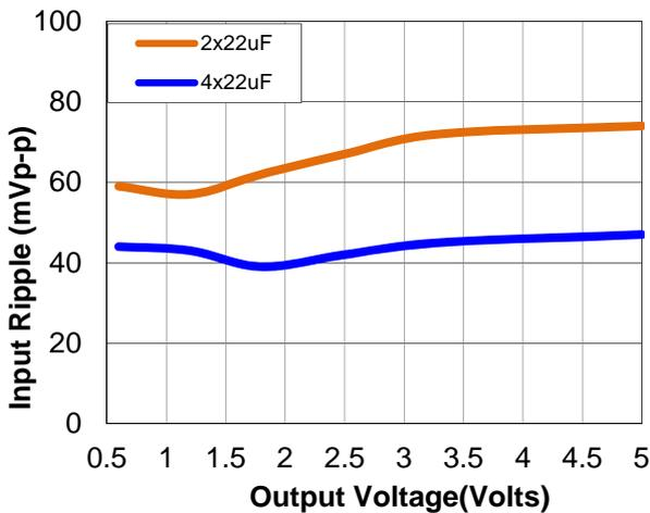
**Figure 37. Input ripple voltage for various output voltages with 2x22  $\mu$ F or 4x22  $\mu$ F ceramic capacitors at the input (2 x 6A load). Input voltage is 12V. Scope BW: 20MHz**
