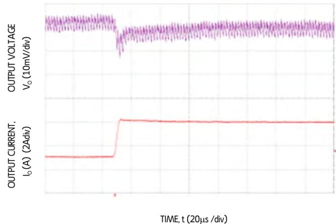
Figure 4. Transient Response to Dynamic Load Change from 50% to 100% on one output at 12Vin,  $C_{out} = 3 \times 47\mu F + 3 \times 330\mu F$ ,  $C_{Tune} = 12nF$ ,  $R_{Tune} = 300$
