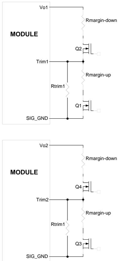
Figure 43. Circuit Configuration for margining Output voltage.
