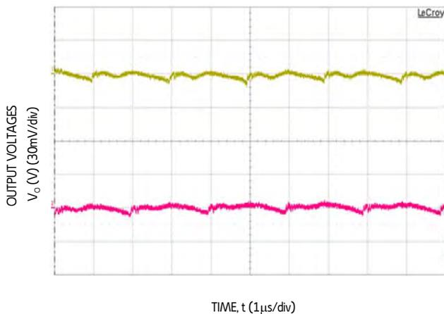
Figure 3. Typical output ripple and noise ( $C_o = 2 \cdot 4.7nF + 2 \cdot 47\mu F$  ceramic,  $V_{IN} = 12V$ ,  $I_o = I_{o1,max}, I_{o2,max}$ ).
