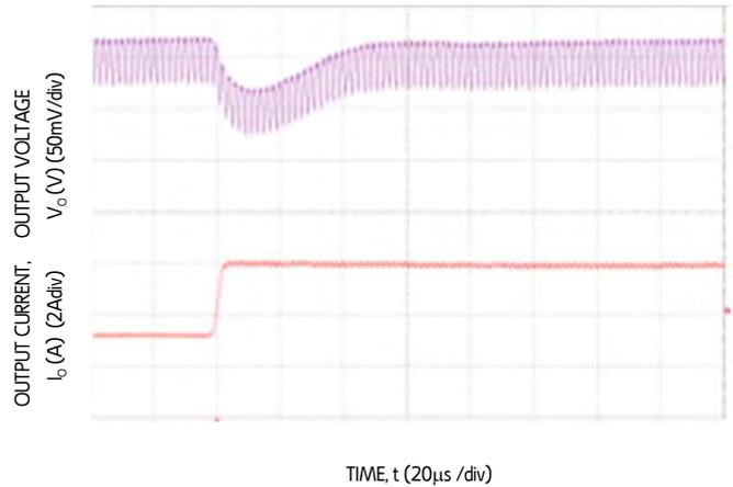
Figure 28. Transient Response to Dynamic Load Change on one output from 50% to 100% at 12V<sub>in</sub>,  $C_{out} = 2 \times 47\mu F + 1 \times 330\mu F$ ,  $C_{Tune} = 1200pF$  &  $R_{Tune} = 300$
