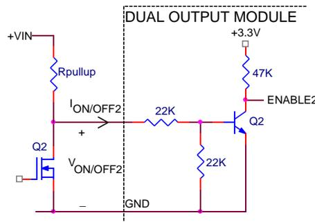
Figure 40. Circuit configuration for using negative On/Off logic.
