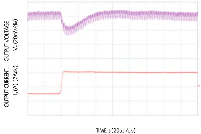
Figure 10. Transient Response to Dynamic Load Change on one output from 50% to 100% at 12Vin,  $C_{out} = 3 \times 47\mu\text{F} + 2 \times 330\mu\text{F}$ ,  $C_{Tune} = 2700\text{pF}$  &  $R_{Tune} = 300$
