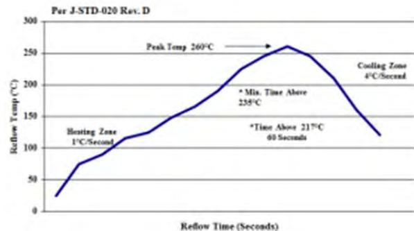
Figure 51. Recommended linear reflow profile using Sn/Ag/Cu solder.
