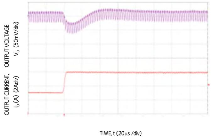
Figure 22. Transient Response to Dynamic Load Change on one output from 50% to 100% at 12Vin,  $C_{out} = 2 \times 47\mu F + 1 \times 330\mu F$ ,  $C_{Tune} = 1500pF$  &  $R_{Tune} = 300$
