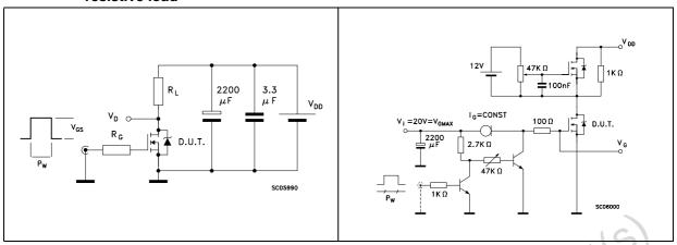
Figure 16. Test circuit for inductive load switching and diode recovery times
