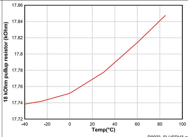
**Figure 7-21. Thermistor Pullup Resistance vs. Temperature (18-kΩ setting)**
