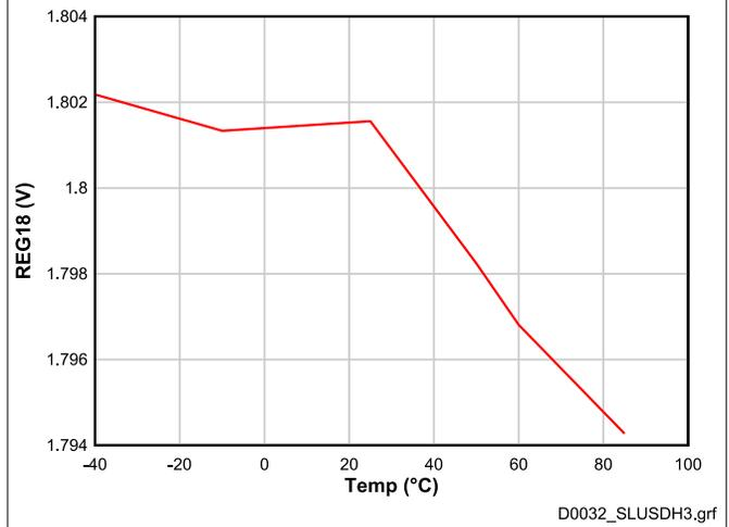
**Figure 7-25. REG18 Voltage vs. Temperature, with No Load**
