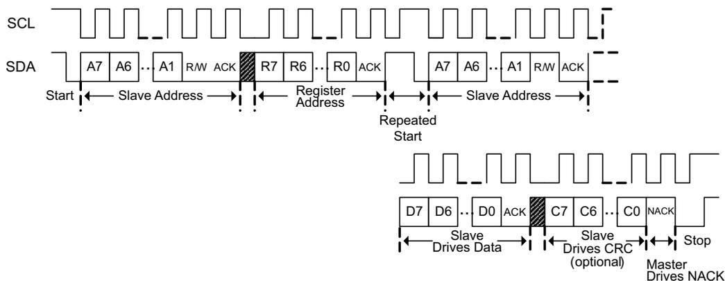
**Figure 14-2. I<sup>2</sup>C Read with Repeated Start**
