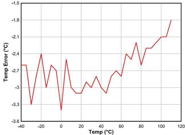
Measurements taken using Semitec 103-AT thermistor, default temperature polynomial, and 18-kΩ internal pullup resistor.
