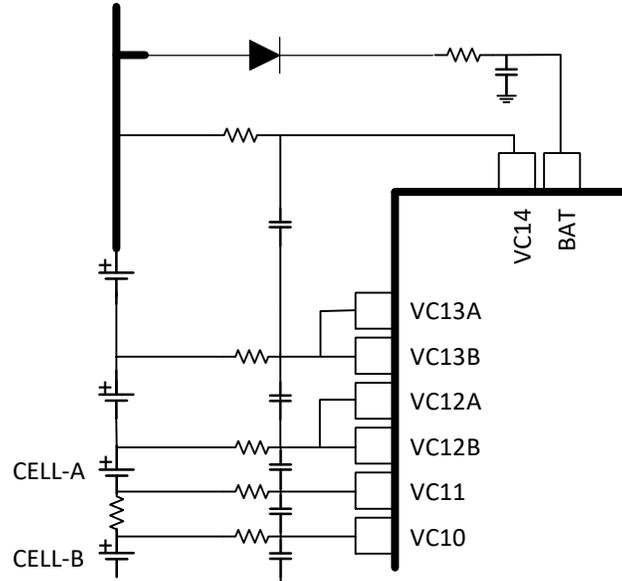
**Figure 10-1. Using Cell Input Pins for Interconnect Measurement**
