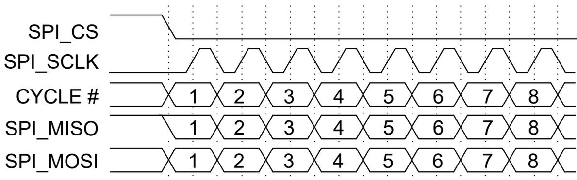
Figure 14-4. SPI with CPOL = 0 and CPHA = 0
