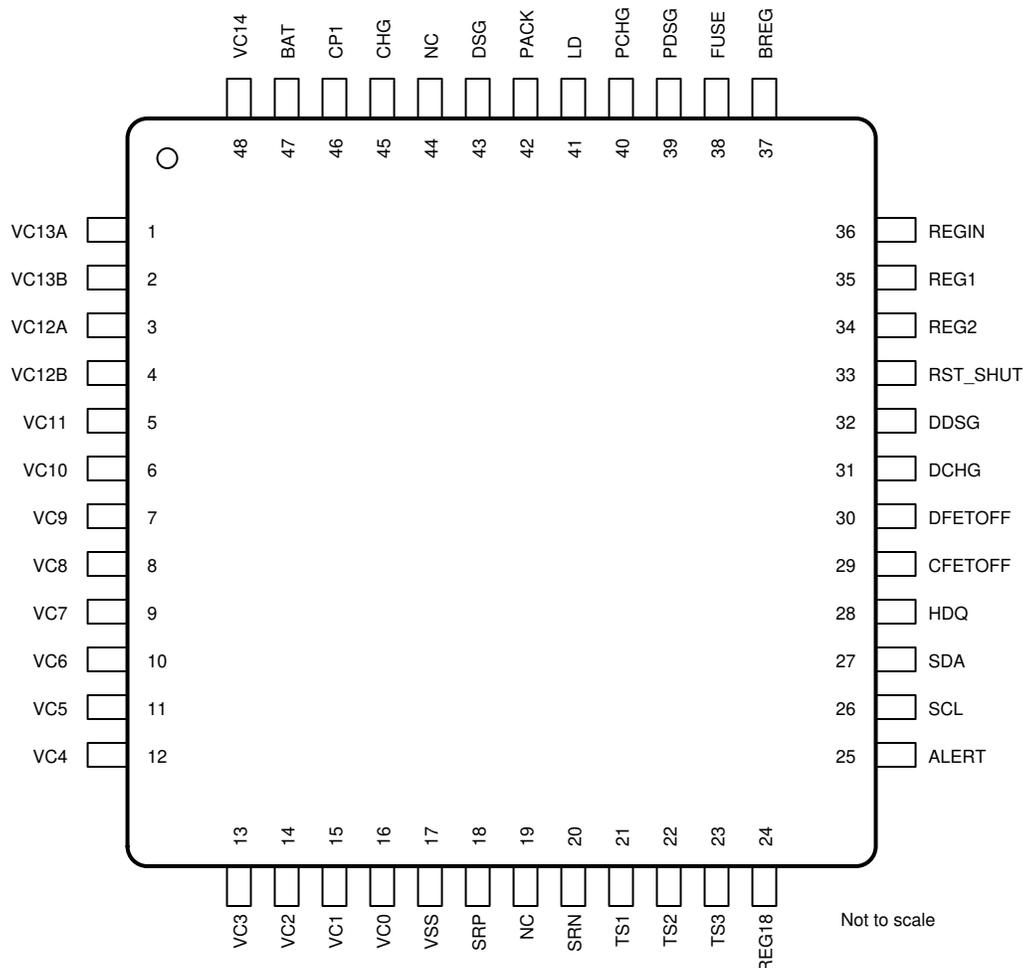
Table 6-1. BQ769142 TQFP Package (PFB) Pin Functions
