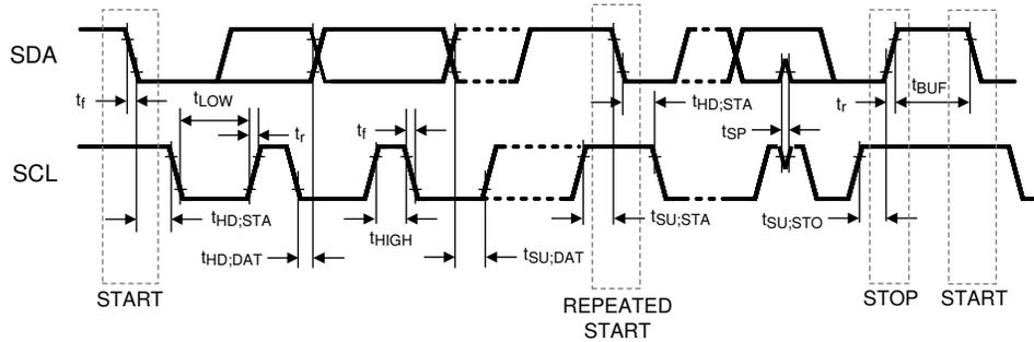
**Figure 7-1. I<sup>2</sup>C Communications Interface Timing**
