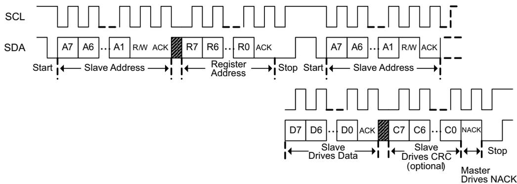
Figure 14-3. I<sup>2</sup>C Read Without Repeated Start
