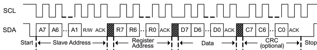
**Figure 14-1. I<sup>2</sup>C Write**
