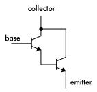
In the Darlington configuration, the emitter of one transistor is hooked to the base of another. This effectively makes one new "super transistor" out of the two, since it is the amplified current out of the first collector that serves as the base current for the second transistor. If the gain of a single transistor were 30, then the effective gain of the Darlington pair would be  $30 \times 30 = 900$ .
