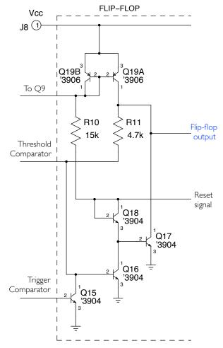
Figure 7: Flip Flop Block
