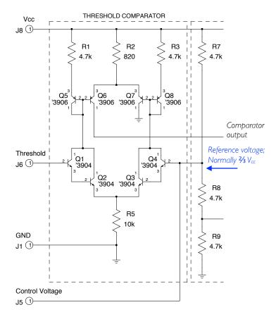
Figure 3: Threshold Comparator
