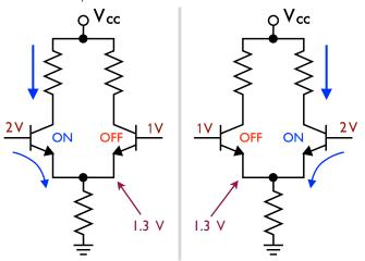
Figure 4: Simplified differential amplifier
