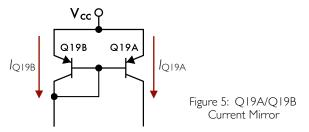
Notice that transistor Q19B is connected "as a diode," with its base short-circuited to its collector. Even so, it allows current to pass through its collector.
