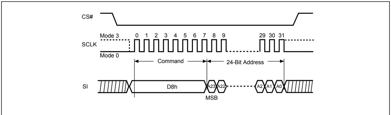
**Figure 44. Block Erase (BE) Sequence (QPI Mode)**
