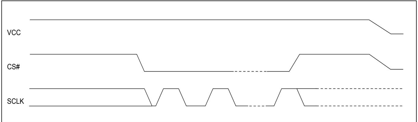
**Figure 86. Power-up Timing**
