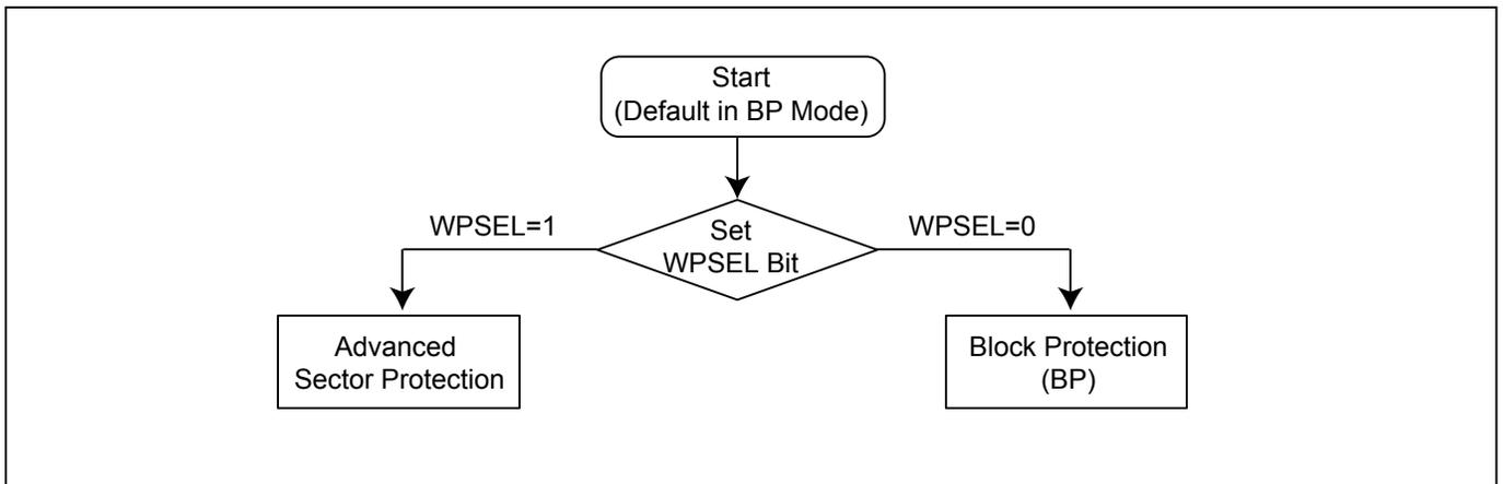
**Figure 61. WPSEL Flow**
