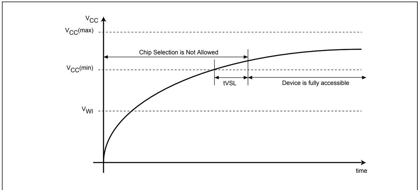
**Figure 87. Power Up/Down and Voltage Drop**
