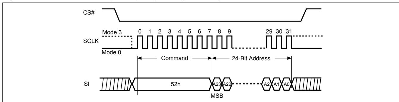
**Figure 42. Block Erase 32KB (BE32K) Sequence (QPI Mode)**
