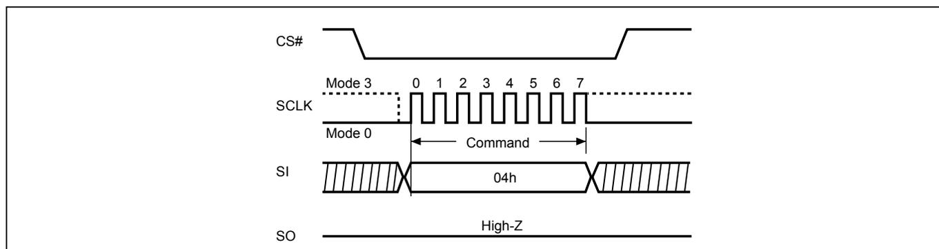
**Figure 9. Write Disable (WRDI) Sequence (QPI Mode)**
