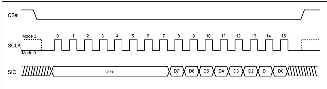
**Figure 36. Burst Read (QPI Mode)**
