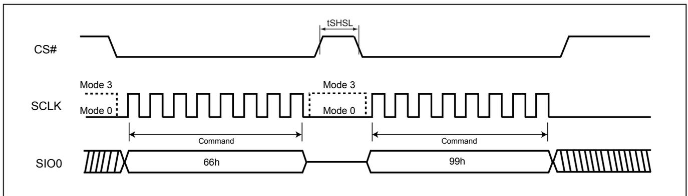
**Figure 76. Reset Sequence (QPI mode)**
