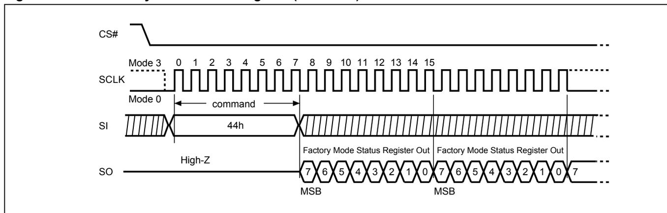
**Figure 53. Read Status Register (RDSR) Sequence (QPI Mode)**
