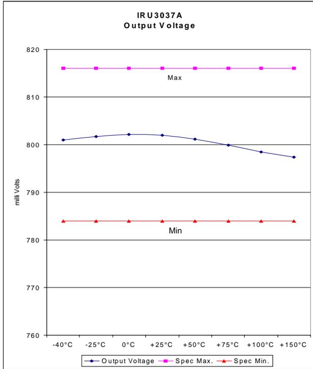
Figure 14 - Output Voltage
