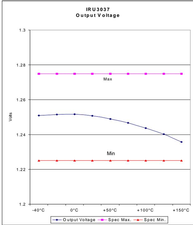
Figure 11 - Output Voltage
