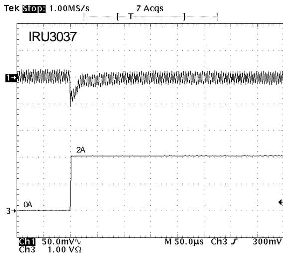
Figure 25 - Transient response @ IOUT= 0 to 2A.
