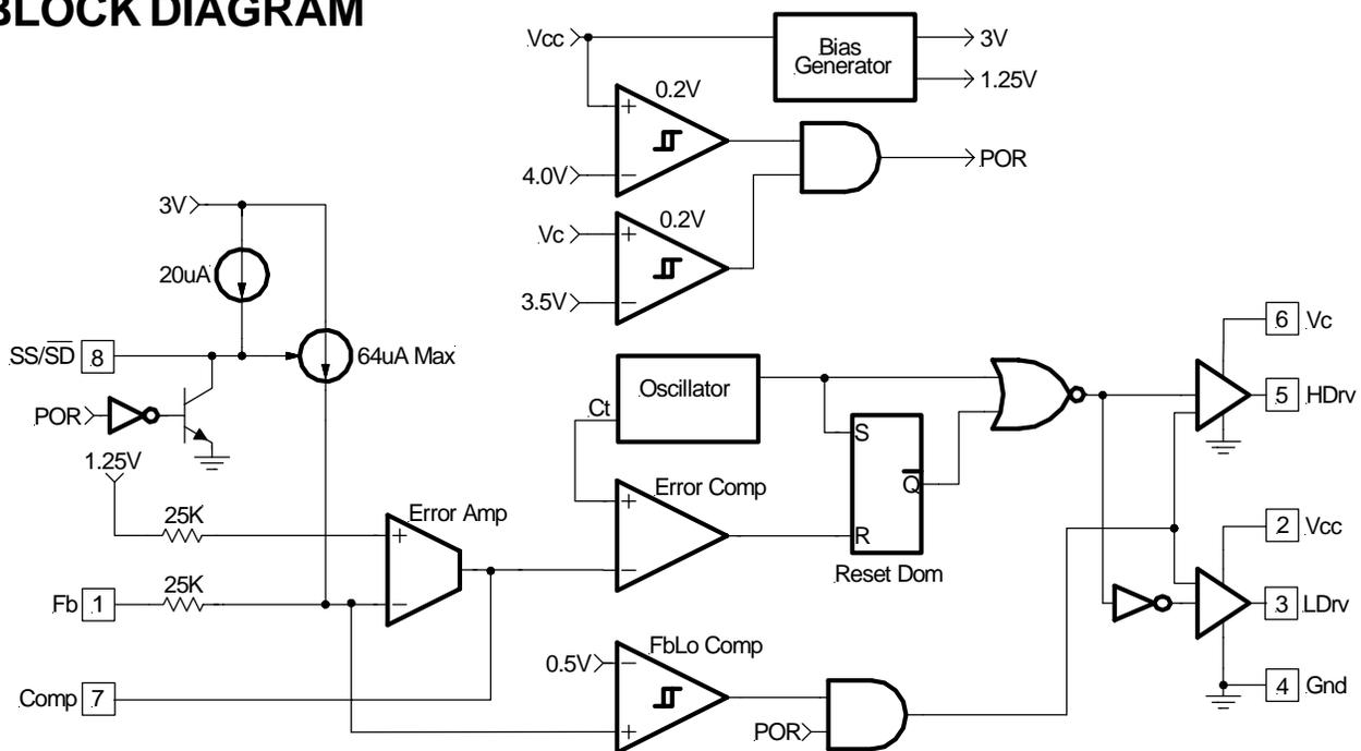
Figure 2 - Simplified block diagram of the IRU3037.
