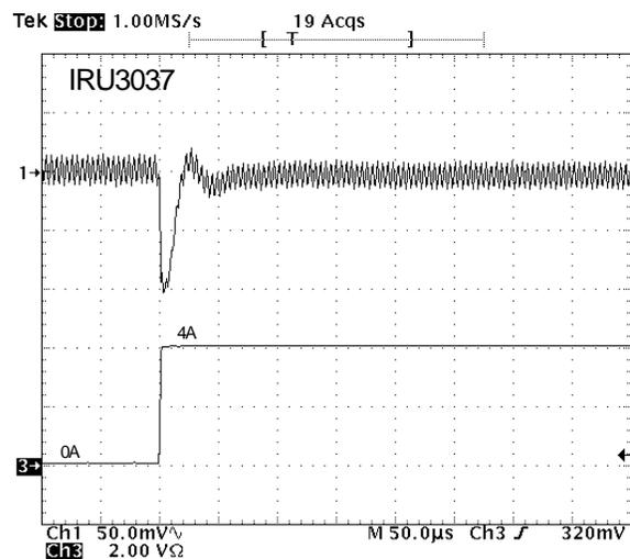
Figure 26 - Transient response @ IOUT= 0 to 4A.
