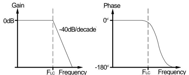
Figure 5 - Gain and phase of LC filter.
