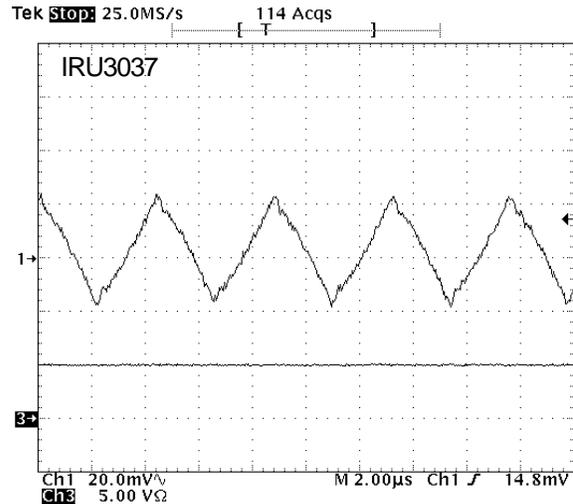
Figure 24 - 3.3V output voltage ripple @ IOUT=5A.
