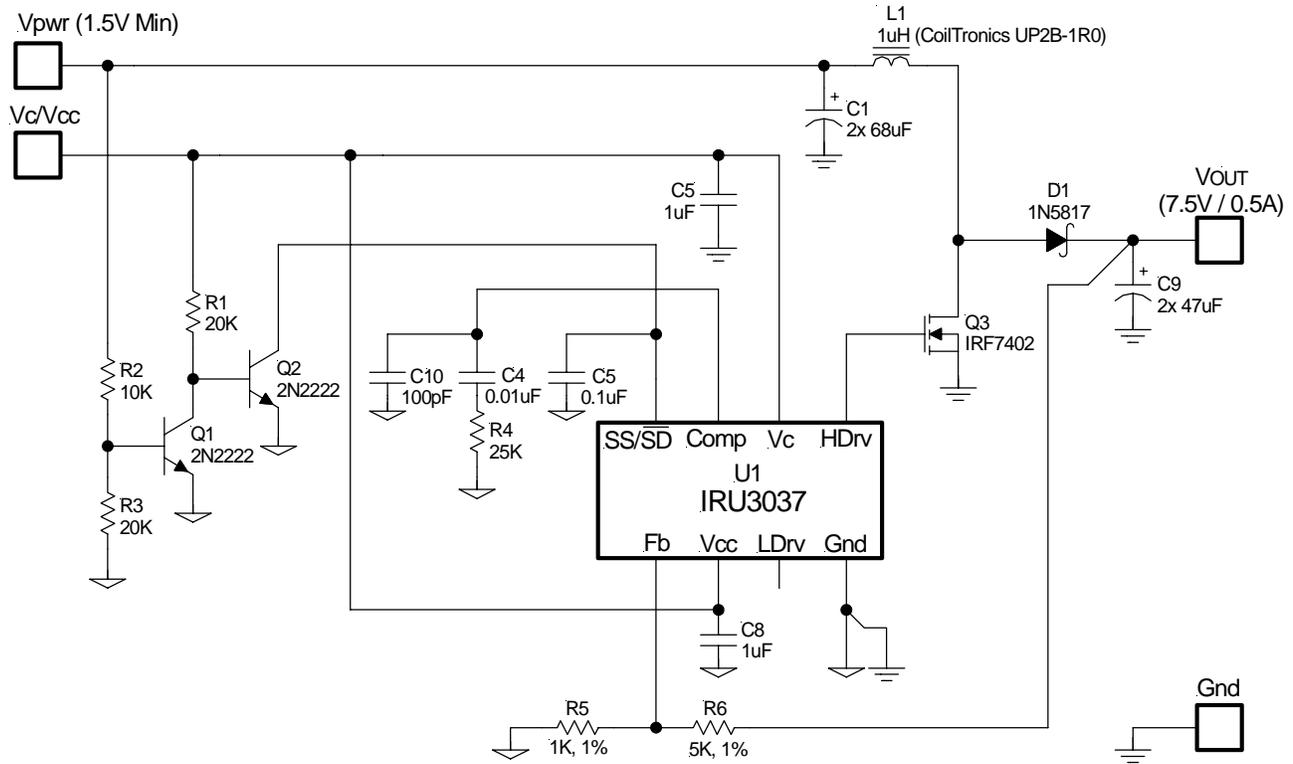
Figure 19 - Typical application of IRU3037 as a boost converter.
