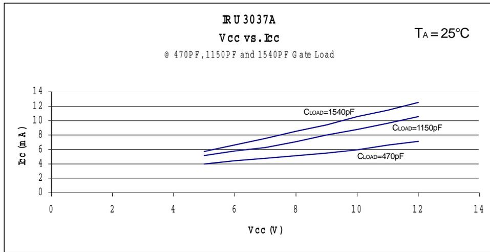
Figure 9 - V<sub>CC</sub> vs. I<sub>CC</sub>
