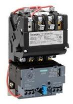
Non-reversing motor starter Size 0 Three phase full voltage Solid-state overload relay OLRelay amp range 3-12A 220-240/440-480VAC 60HZ coil Combination type No enclosure
