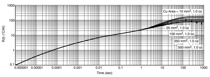
Figure 47. Transient Thermal Response Simulation to a Single Pulse 1 oz (Log-Log)
