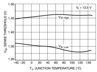
Figure 32. Sense Threshold vs. Junction Temperature
