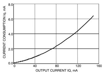
Figure 12. Current Consumption Iq vs. Output Current IQ
