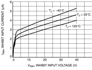
Figure 29. Inhibit Input Current at Inhibit Input Voltage Extremes
