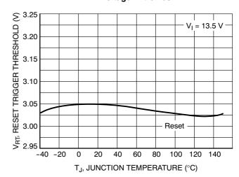
Figure 30. Reset Trigger Threshold vs. Junction Temperature
