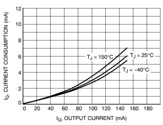
Figure 20. Current Consumption vs. Output
