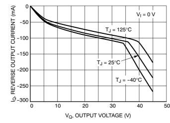
Figure 23. Reverse Output Current vs. Output Voltage
