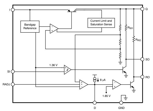
Figure 1. SO-8 Simplified Block Diagram
