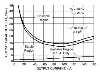
Figure 18. Stability vs. Output Capacitor ESR
