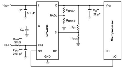
$<sup>{}^{\</sup>star}C_{l}$  required if regulator is located far from the power supply filter.
