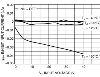
Figure 28. Inhibit Input Current at Input Voltage Extremes
