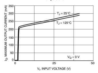
Figure 24. Maximum Output Current vs. Input Voltage
