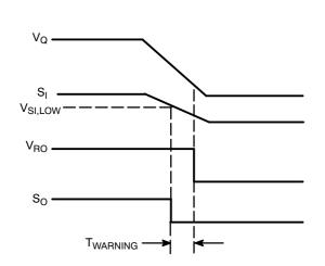
Figure 42. SO Warning Timing Waveform
