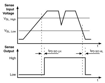
Figure 43. Sense Timing Diagram
