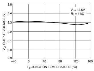
Figure 22. Output Voltage vs. Junction Temperature
