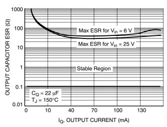
Figure 26. 3.3 V Output Stability with Output Capacitor ESR
