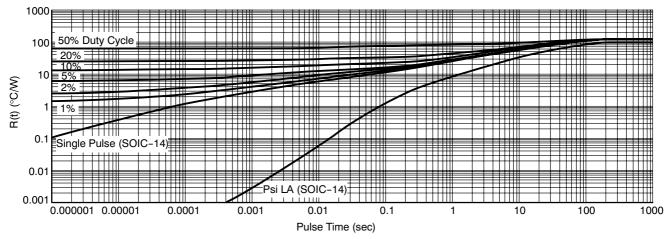
Figure 48. Transient Thermal Response Simulation to a Single Pulse with Duty Cycles Applied (Log-Log) (PCB = 50 mm<sup>2</sup> 1 oz)
