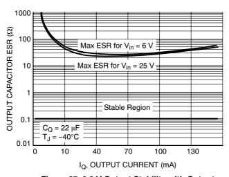
Figure 27. 3.3 V Output Stability with Output Capacitor ESR
