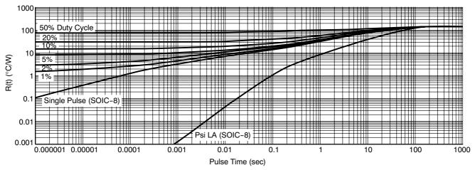
Figure 46. Transient Thermal Response Simulation to a Single Pulse with Duty Cycles Applied (Log-Log) (PCB = 250 mm<sup>2</sup> 1 oz)
