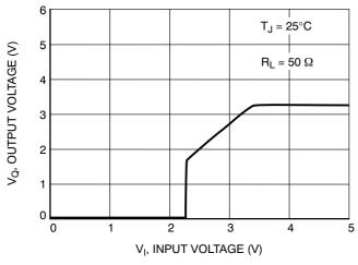
Figure 25. Output Voltage at Input Voltage Extremes
