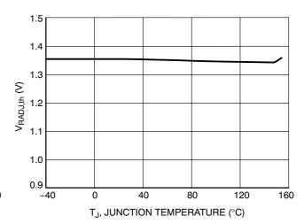
Figure 36. Reset Adjust Switching Threshold vs. Junction Temperature
