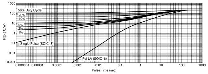
Figure 45. Transient Thermal Response Simulation to a Single Pulse with Duty Cycles Applied (Log-Log) (PCB = 50 mm<sup>2</sup> 1 oz)
