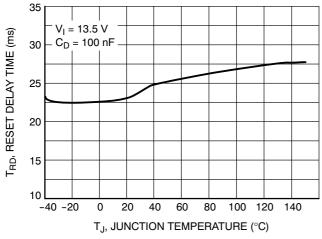
Figure 31. Reset Delay Time vs. Junction Temperature
