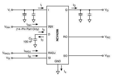
Figure 3. Measurement Circuit
