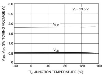
Figure 35. Switching Voltage  $V_{UD}$  and  $V_{LD}$  vs. Junction Temperature
