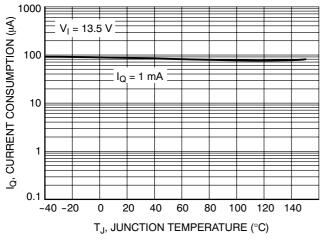
Figure 19. Current Consumption vs. Junction Temperature
