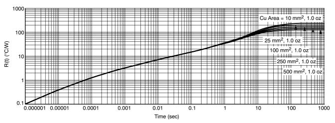
Figure 44. Transient Thermal Response Simulation to a Single Pulse 1 oz (Log-Log)
