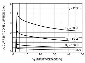
Figure 21. Current Consumption vs. Input Voltage
