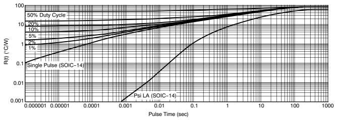
Figure 49. Transient Thermal Response Simulation to a Single Pulse with Duty Cycles Applied (Log-Log) (PCB = 250 mm<sup>2</sup> 1 oz)
