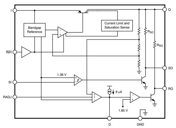
Figure 2. SO-14 Simplified Block Diagram
