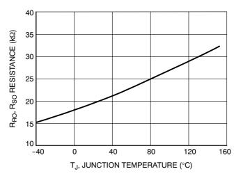
Figure 38. R<sub>RO</sub>, R<sub>SO</sub> Resistance vs. Junction Temperature
