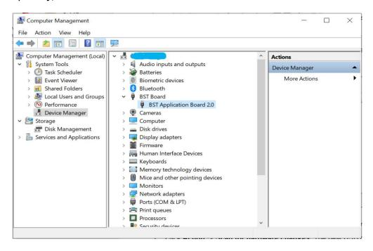
Figure 21: Selecting USB device corresponding to application board
