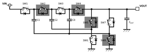
Figure 19-A. Divide by Four Charge Pump Phase One Configuration
