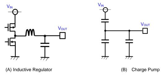
Figure 30. Inductive Regulator and Charge Pump
