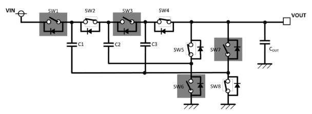
Figure 19-B. Divide by Four Charge Pump Phase Two Configuration
