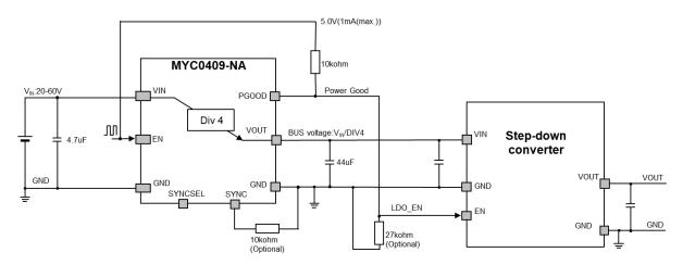
Figure 27. Application Schematic with Secondary
