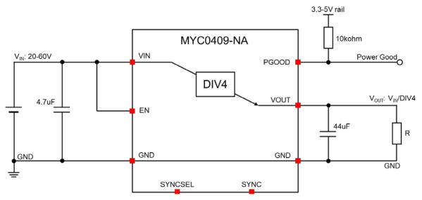
Figure 6. Application Circuit
