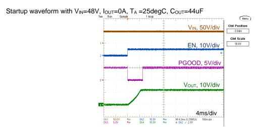
Figure 8. Start-up Waveform
