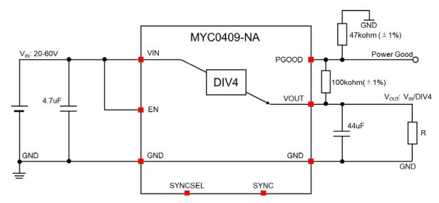
Figure 17. PGOOD Application Circuit
