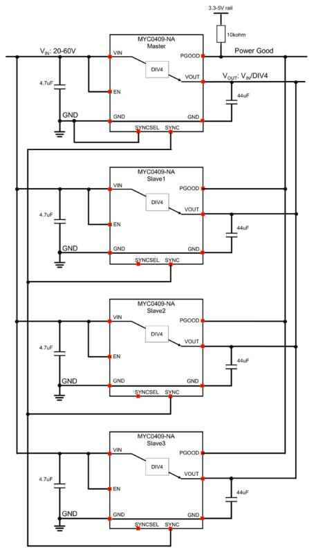
Figure 29. Multi-module Application Circuit
