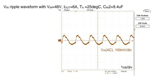
Figure 11. V<sub>IN</sub> Ripple Waveform
