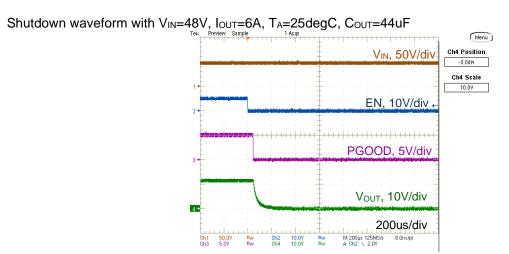
Figure 9. Shutdown Waveform
