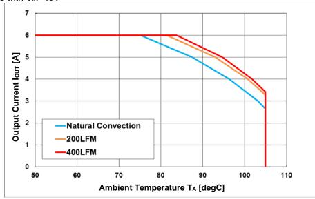
Figure 13. Thermal Deratings (V<sub>IN</sub>=48V)
