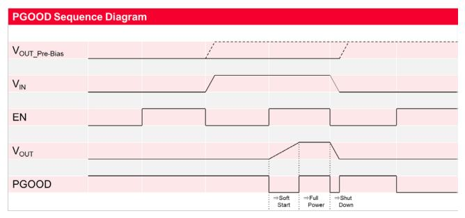
Figure 16. PGOOD Sequence Diagram
