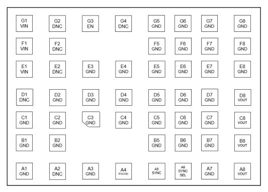
Figure 4. Module Terminals (Top View)
