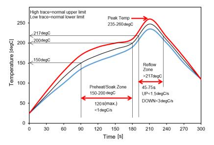
Figure 38. Reflow Profile for Sn/Ag/Cu Solder
