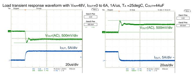
Figure 12. Load Transient Response Waveform
