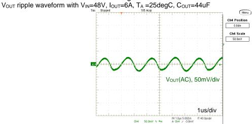
Figure 10. Vout Ripple Waveform
