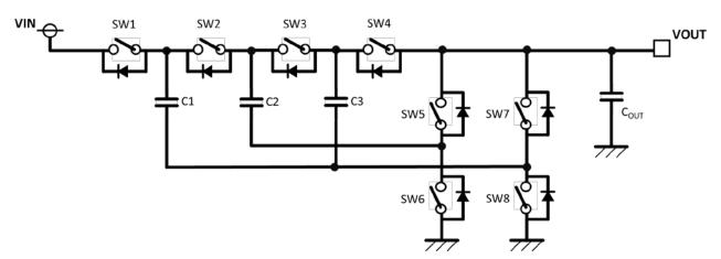
Figure 18. Divide by Four Charge Pump Configuration
