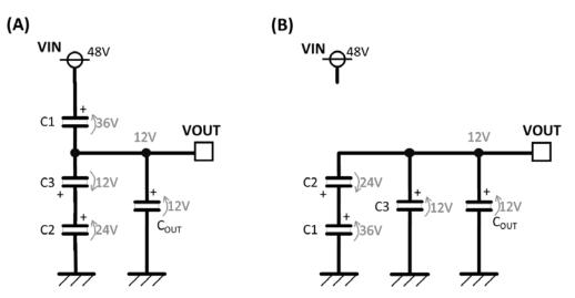
Figure 20. Divide by Four Charge Pump Capacitor Connection
