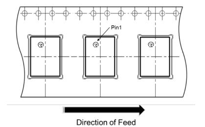
Figure 36. Module Orientation in Tape
