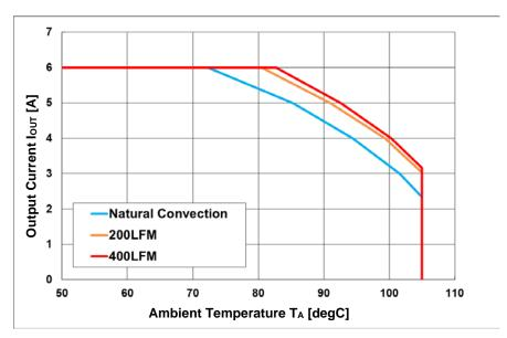
Figure 14. Thermal Deratings (V<sub>IN</sub>=54V)
