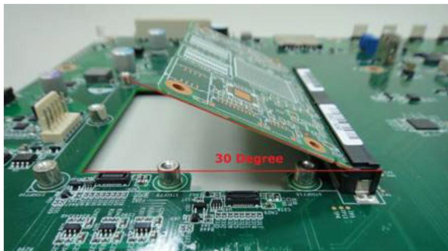
2. Press down the module board and make sure the 4 screw holes are aligned with the carrier board and adjust the 4 screws clockwise to fix them in place
