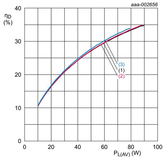
$V_{DS} = 32\text{ V}; I_{Dq} = 1700\text{ mA}$ .
