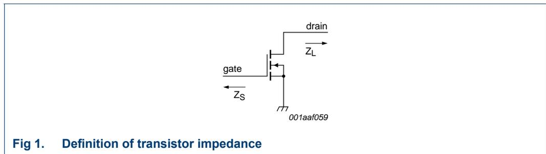
**Fig 1. Definition of transistor impedance**
