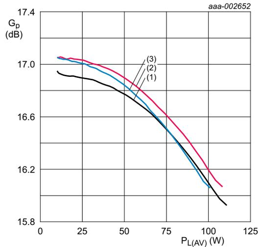
$V_{DS} = 32\text{ V}$ ;  $I_{Dq} = 1700\text{ mA}$ ; channel spacing = 5 MHz;
