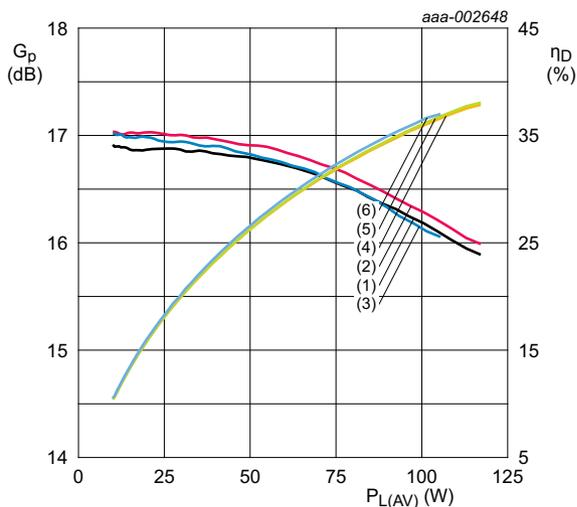
$V_{DS} = 32\text{ V}$ ;  $I_{DQ} = 1700\text{ mA}$ ;  $PAR = 7.2\text{ dB}$  at 0.01 % probability on the CCDF.
