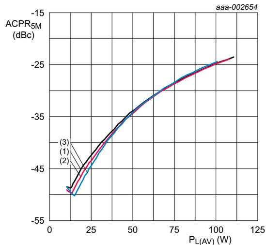
$V_{DS} = 32\text{ V}$ ;  $I_{Dq} = 1700\text{ mA}$ ; channel spacing = 5 MHz;
