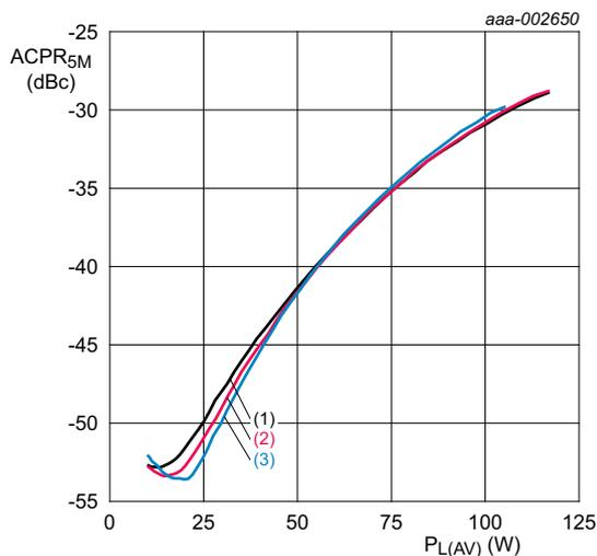
$V_{DS} = 32\text{ V}$ ;  $I_{DQ} = 1700\text{ mA}$ ;  $PAR = 7.2\text{ dB}$  at 0.01 % probability on the CCDF.
