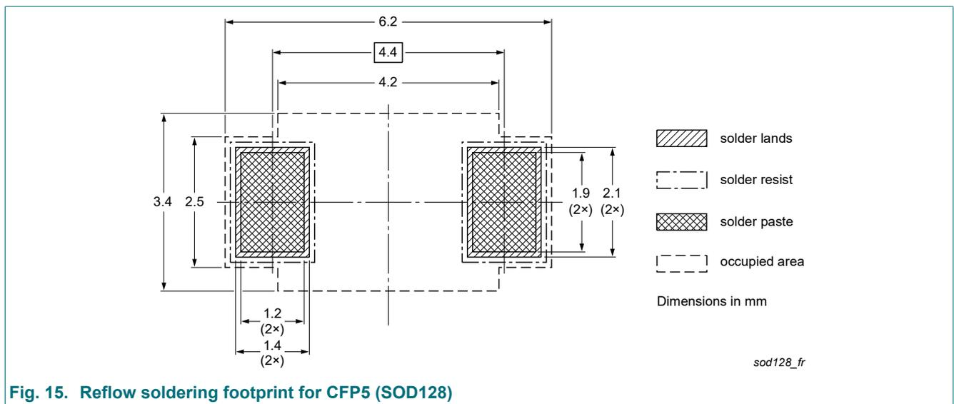
Fig. 15. Reflow soldering footprint for CFP5 (SOD128)
