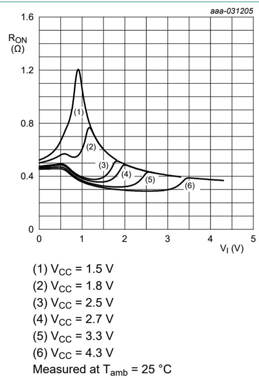
Fig. 7. Typical ON resistance as a function of input voltage
