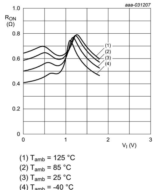
Fig. 9. ON resistance as a function of input voltage; V<sub>CC</sub> = 1.8 V
