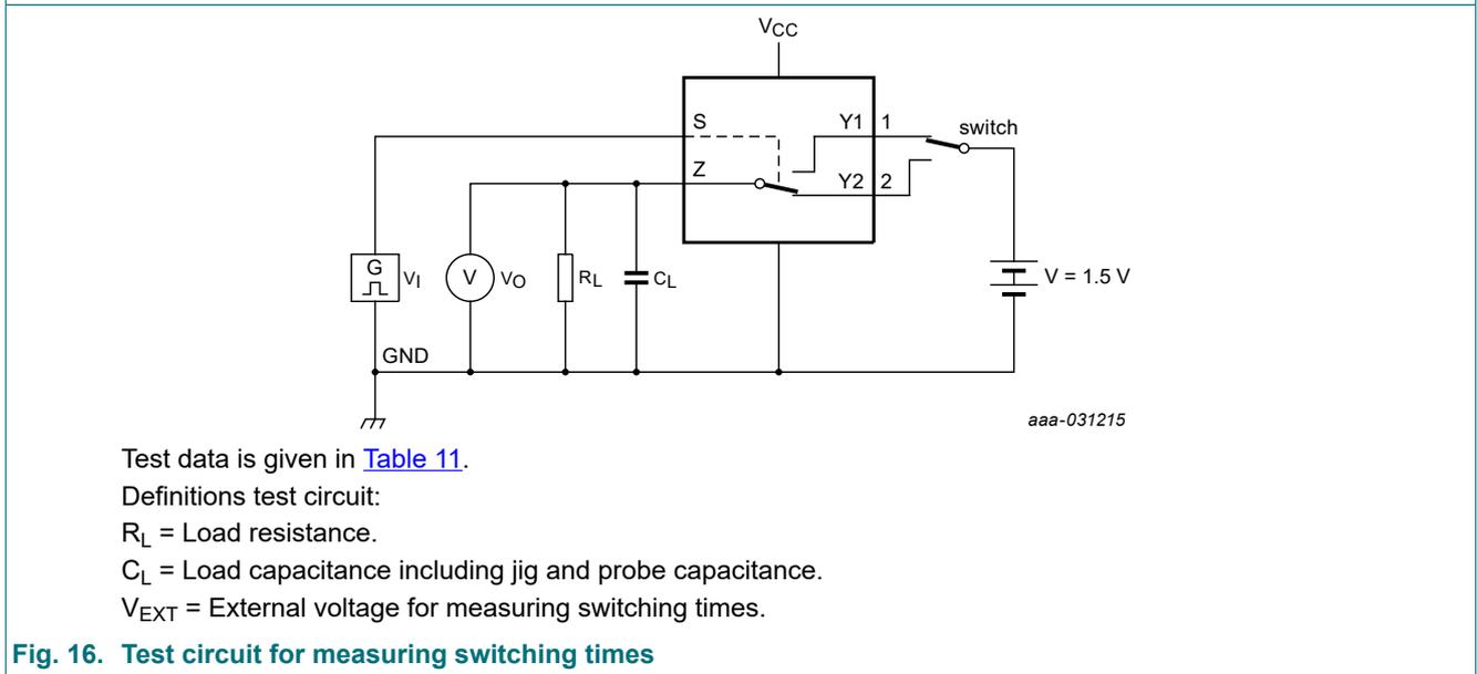
Fig. 16. Test circuit for measuring switching times
