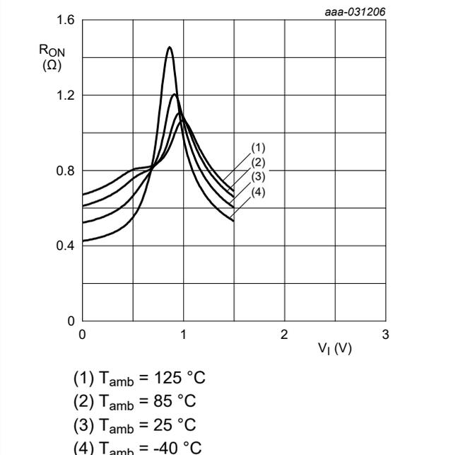
Fig. 8. ON resistance as a function of input voltage; V<sub>CC</sub> = 1.5 V
