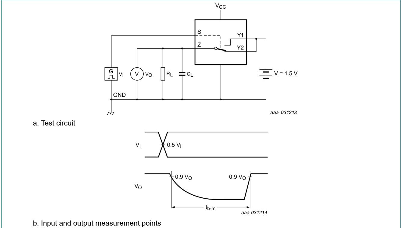
Fig. 15. Test circuit for measuring break-before-make times
