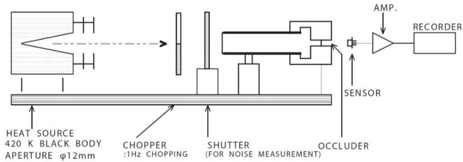
**Figure 2 - Occluder Position**
