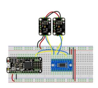
Board 3V to mux VIN (red wire)
