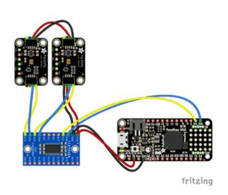
Board 3V to mux VIN (red wire)
