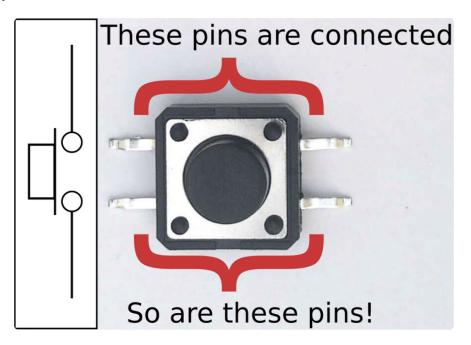
So don't forget when using in the breadboard that the two rows across from each other will be connected on the inside of the switch!
