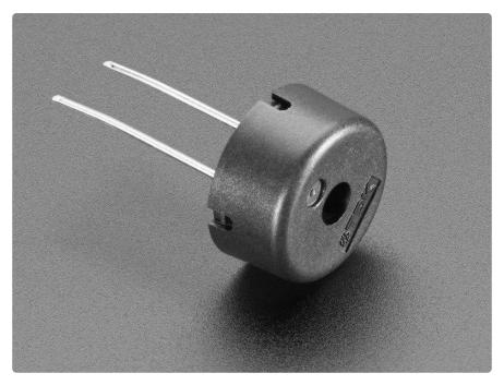
Piezo buzzers are used for making beeps, tones and alerts. Its the same thing that's in your microwave, alarm clock or washing machine to alert you when your food is done, or laundry complete. This one is petite but loud! You can plug it into your breadboard easily. Drive it with square wave to make tones - that's it, pretty easy.
