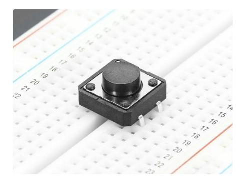
The switches have four legs, but there's only two halves to the switch. The two sets of pins are normally open (disconnected) and when the button is pressed they are momentarily closed.
