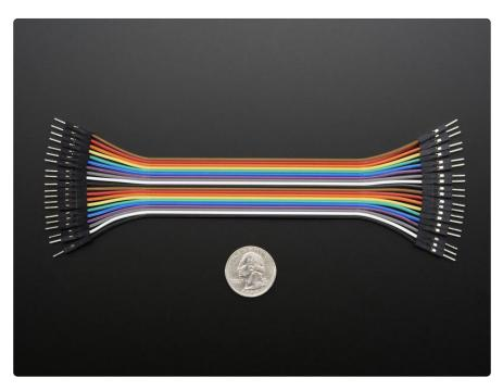
Each version comes in a 'strip' of 20 (2 pieces of each of ten rainbow colors). They have 0.1" male header contacts on either end and fit cleanly next to each other on standard-pitch 0.1" (2.54mm) breadboards. The best part is they come in a 20-pin
