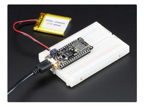
If the battery is plugged into the Feather and the USB cable is connected to a computer or power supply it will automatically recharge the battery. The yellow LED will light up to let you know. When the yellow light turns off, the battery is done charging
