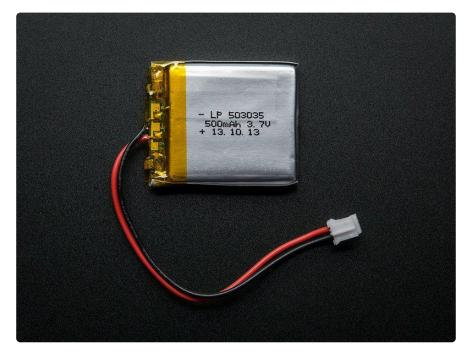
Lithium ion polymer (also known as 'lipo' or 'lipoly') batteries are thin, light and powerful. The output ranges from 4.2V when completely charged to 3.7V. This battery has a capacity of 500mAh for a total of about 1.9 Wh.
