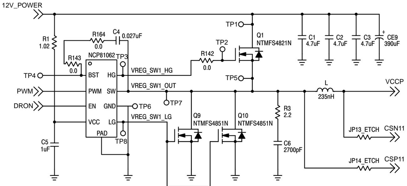
Figure 3. Application Circuit
