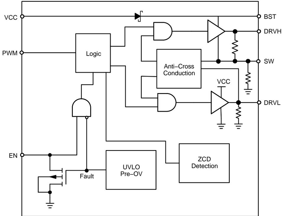
Figure 2. Block Diagram
