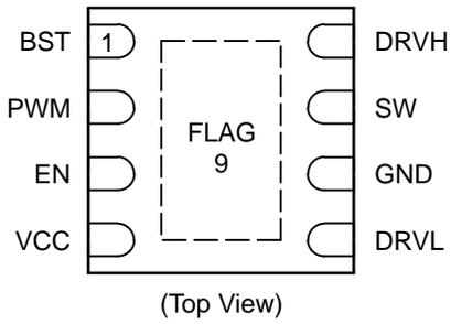
Figure 1. Pin Diagram
