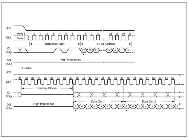
Figure 10. Fast Read Instruction Sequence Diagram
