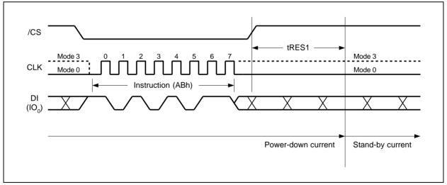
Figure 28a. Release Power-down Instruction Sequence
