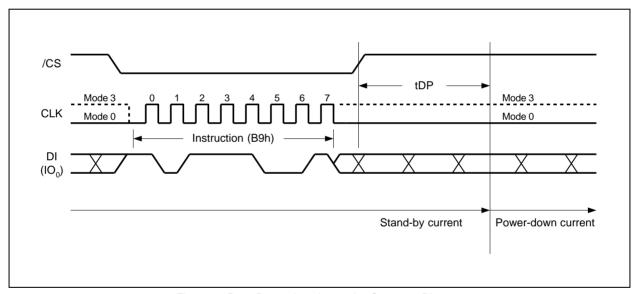
Figure 27. Deep Power-down Instruction Sequence Diagram
