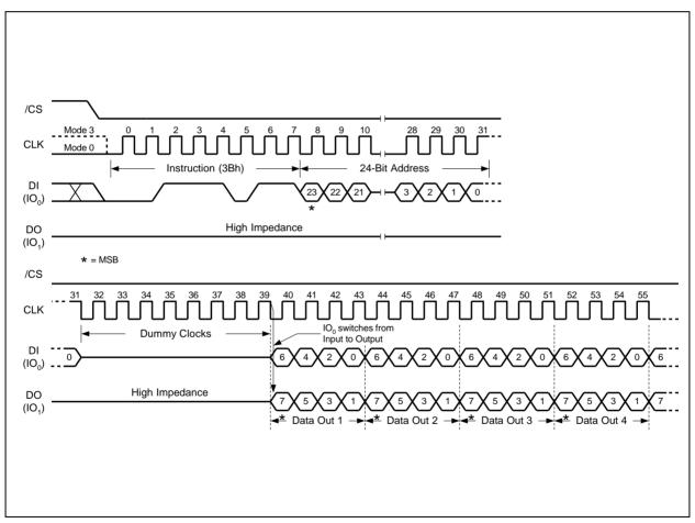
Figure 11. Fast Read Dual Output Instruction Sequence Diagram
