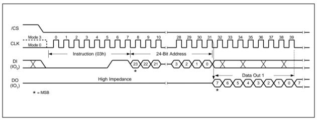
Figure 9. Read Data Instruction Sequence Diagram
