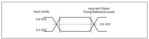
Figure 38. AC Measurement I/O Waveform
