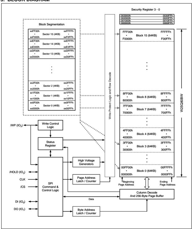
Figure 2. W25Q80BW Serial Flash Memory Block Diagram
