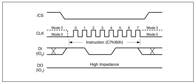
Figure 24. Chip Erase Instruction Sequence Diagram
