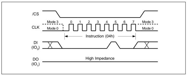
Figure 6. Write Disable Instruction Sequence Diagram
