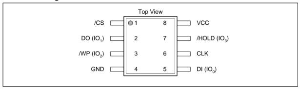
Figure 1a. W25Q80BW Pin Assignments, 8-pin SOIC / VSOP 150 / 208-mil (Package Code SN, SS, SV, ST)
