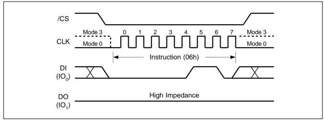
Figure 4. Write Enable Instruction Sequence Diagram
