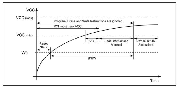
Figure 37. Power-up Timing and Voltage Levels /CS must track VCC during VCC Ramp Up/Down VCC /CS
