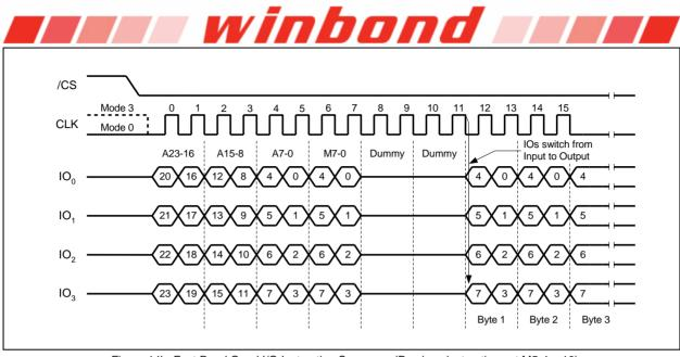
Figure 14b. Fast Read Quad I/O Instruction Sequence (Previous instruction set M5-4 = 10)
