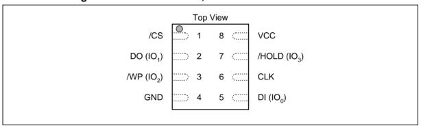
Figure 1b. W25Q80BW Pad Assignments, 8-pad WSON 6x5-mm, USON 4x3-mm (Package Code ZP & UU)
