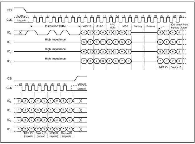
Figure 31. Read Manufacturer / Device ID Quad I/O Diagram
