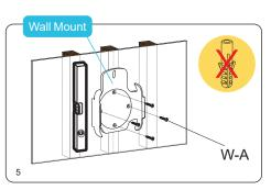
Using a power drill and 5/64" drill bit, drill pilot holes of 5/64" (2mm) diameter and at least 1" (25 mm) depth.
