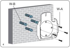
Place concrete anchors (W-B) in each hole. Tap each anchor flush with the wall using a hammer. Mount the wall mount and fasten screws (W-A) using a Phillips screwdriver.
