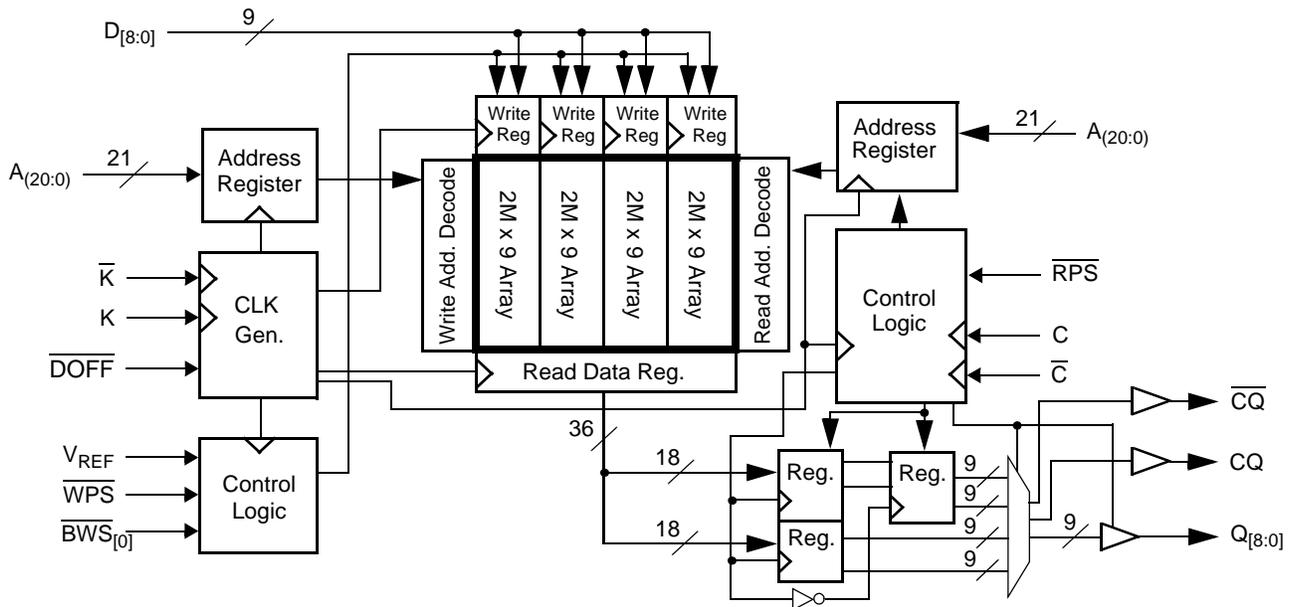
Logic Block Diagram – CY7C1513KV18
