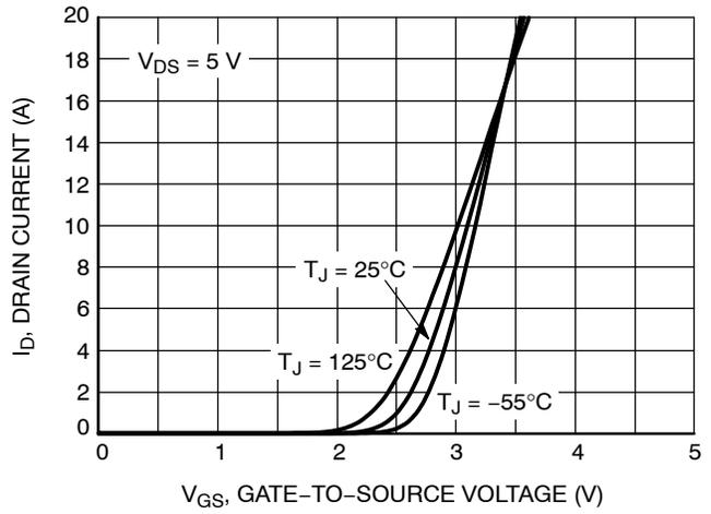
Figure 2. Transfer Characteristics
