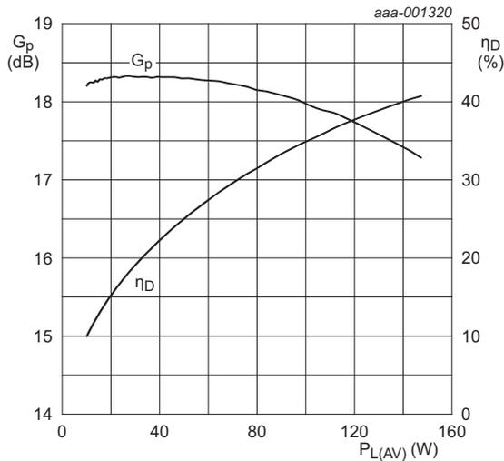
$V_{DS} = 28\text{ V}$ ;  $I_{Dq} = 1900\text{ mA}$ ;  $f = 2140\text{ MHz}$ ;  $PAR = 7.2\text{ dB}$  at 0.01 % probability on the CCDF.
