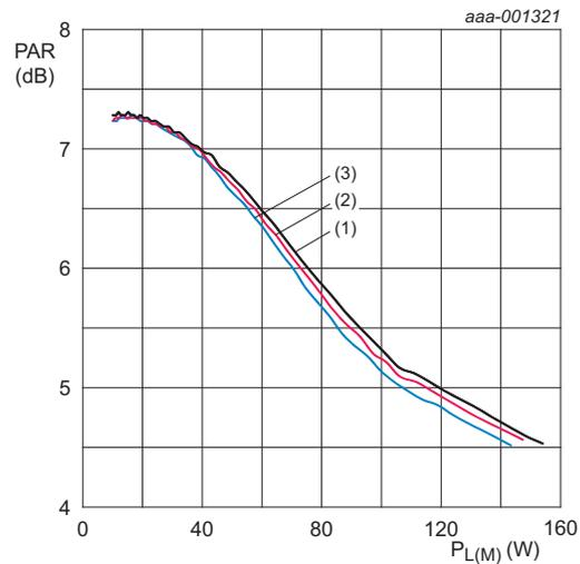
$V_{DS} = 28\text{ V}$ ;  $I_{Dq} = 1900\text{ mA}$ ;  $PAR = 7.2\text{ dB}$  at 0.01 % probability on the CCDF.
