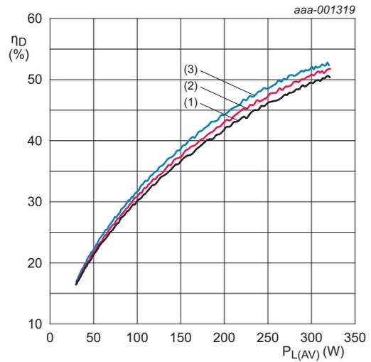
$V_{DS} = 28\text{ V}; I_{Dq} = 1900\text{ mA.}$
