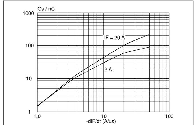
Fig.8. Maximum  $Q_s$  at  $T_j = 25^\circ\text{C}$ ; per diode.
