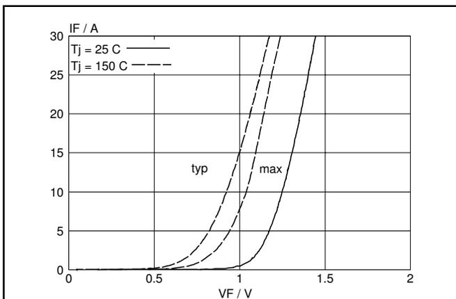
Fig.7. Typical and maximum forward characteristic
