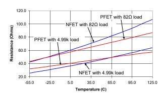
6. Output resistance were measured under the condition of  $V_{CC}$  = +5 V,  $V_{OPT}$  = +5 V, and  $V_{EE}$  = -5 V, with load resistors from outputs to ground.
