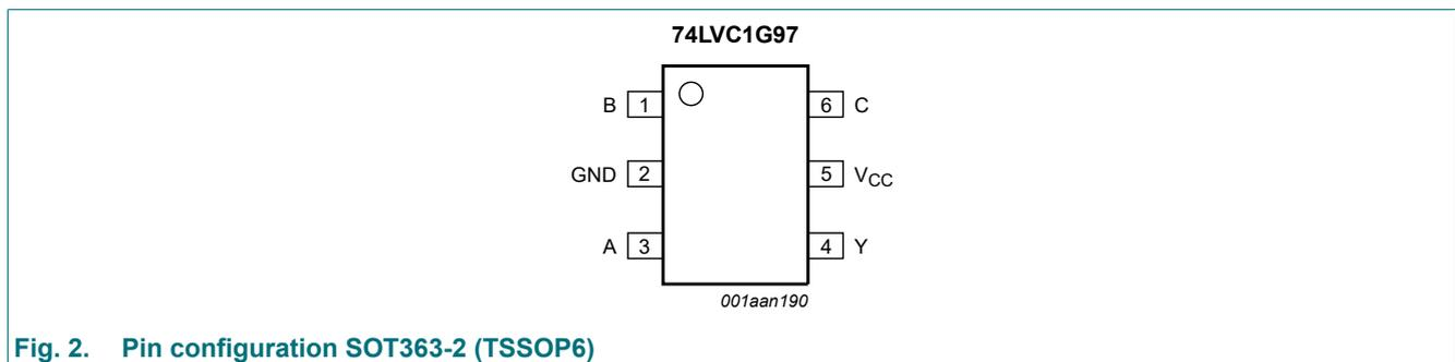
Fig. 2. Pin configuration SOT363-2 (TSSOP6)
