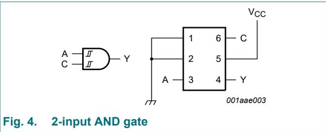
Fig. 4. 2-input AND gate
