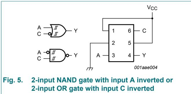
Fig. 5. 2-input NAND gate with input A inverted or 2-input OR gate with input C inverted
