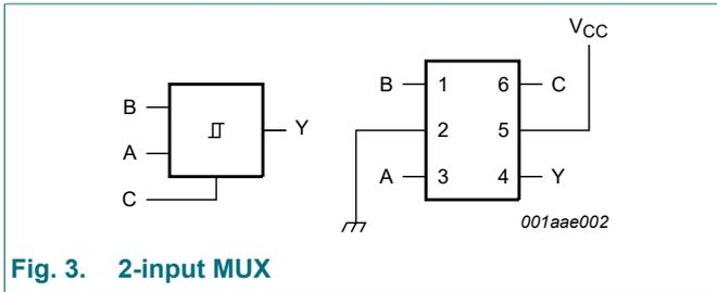
Fig. 3. 2-input MUX
