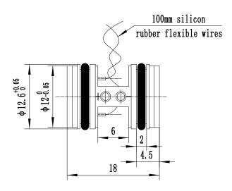
The suggested mounting dimension is  $\Phi 12.6^{+0.12}_{+0.08}$  mm
