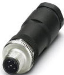
Power connectors, 5-position, Plug straight M12, A-coded, Screw connection, knurl material: Zinc die-cast, nickel-plated, cable gland Pg11, external cable diameter 8 mm ... 10 mm
