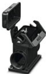
Box mounting bases B16, with single locking latch, material: PA, protective cover material: PA, cable outlets: 2, lateral, height: 84 mm, cable gland: none, support sleeve: no, 2x M25, protective cover: yes, Standard, including 2x reducing adapter
