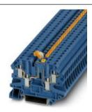
Knife disconnect terminal block, Connection type: Screw connection, Cross section: 0.14 mm² - 6 mm², AWG: 26 - 10, Nominal current: 20 A, Nominal voltage: 500 V, Length: 65.4 mm, Width: 6.2 mm, Color: blue, Assembly: NS 35/7,5, NS 35/15
