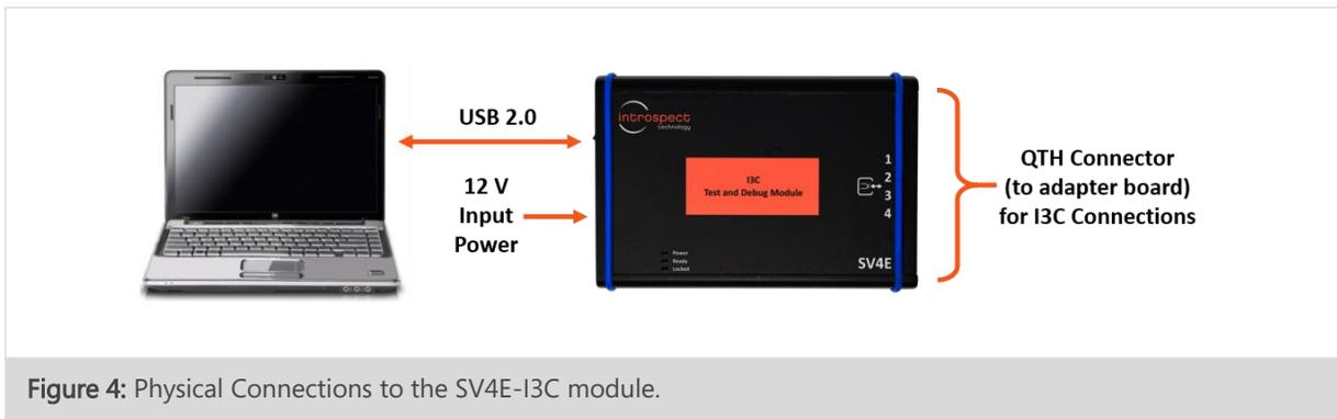
Figure 4: Physical Connections to the SV4E-I3C module.
