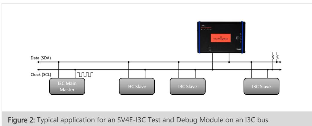
Figure 2: Typical application for an SV4E-I3C Test and Debug Module on an I3C bus.
