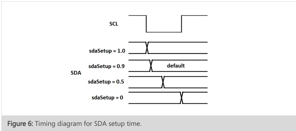
Figure 6: Timing diagram for SDA setup time.
