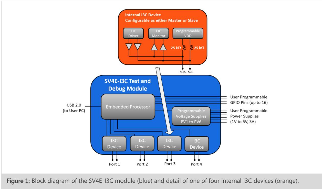
Figure 1: Block diagram of the SV4E-I3C module (blue) and detail of one of four internal I3C devices (orange).
